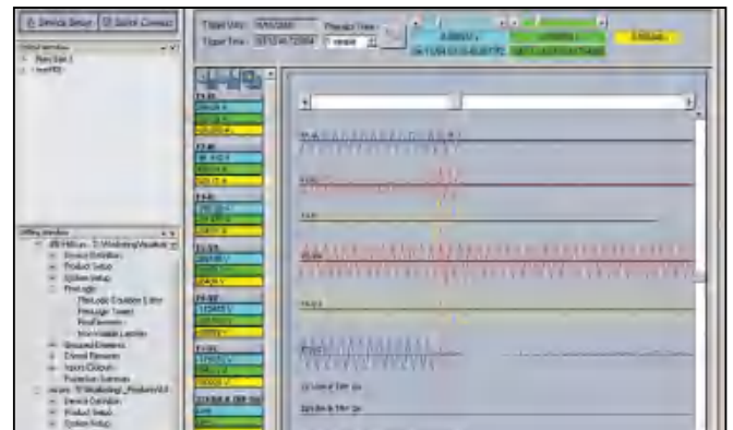
Analyze faults and disturbances using both analog and digital power system quantities.
