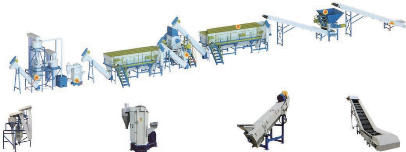
风选系统 Air Classifier 风选集料Cyclone Collection Removes dirt and labels. Collects target materials.
