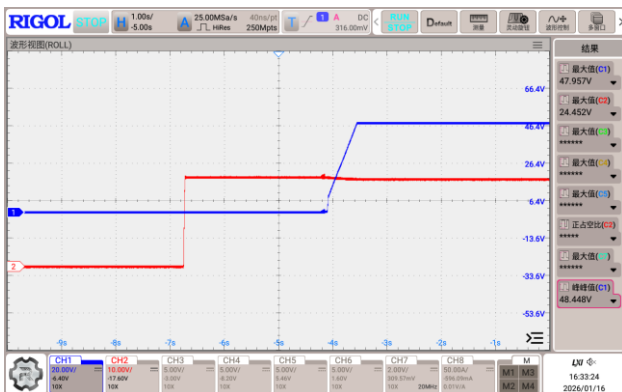
Figure 7, Output voltage established (Iout = 30A)
