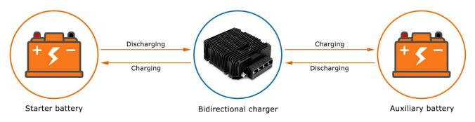
With a WG-24BC900M bidirectional charger, you can charge your dual battery system, and charge your car with the auxiliary battery.
