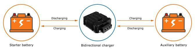
With a WG-12BC900M bidirectional charger, you can charge your dual battery system, and charge your car with the auxiliary battery.
