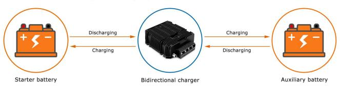
With a WG-36BC900M bidirectional charger, you can charge your dual battery system, and charge your car with the auxiliary battery.
