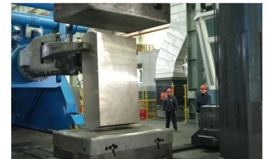
▲ The aluminum plate is ready for forging 铝板准备进行锻造加工
