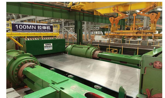
▲ The aluminum plate is being stretched 铝板在进行拉伸加工中
