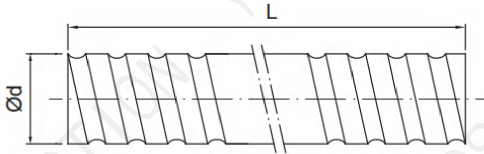
Fig 2.3.1 Screw Shaft Nominal Diameter
