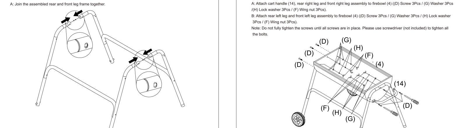
A: Attach wheel (15) onto rear left leg and front left leg ((I) Pin 2Pcs / (J) Cotter pin 2Pcs).
