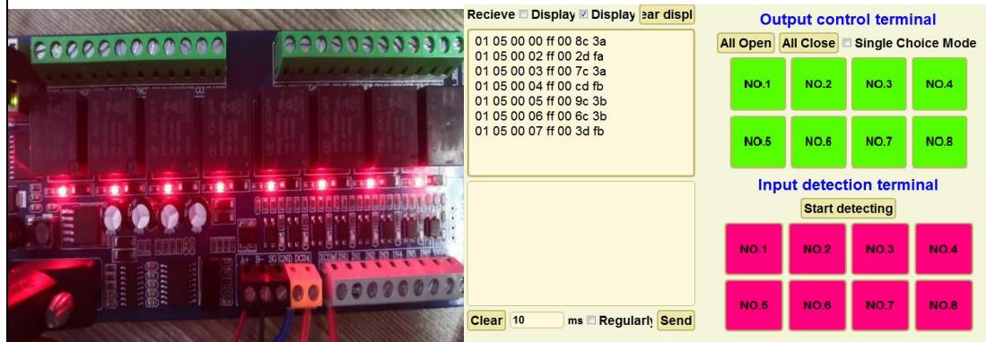
Click "Start Detection" on the input detection terminal, and the 03 code will be sent to the module at a certain time interval, indicating that you want to obtain the current input status, and then judge whether the channel is on or off according to the return code. This time interval varies according to the baud rate, the greater the baud rate, the smaller the time interval. as the picture shows:
