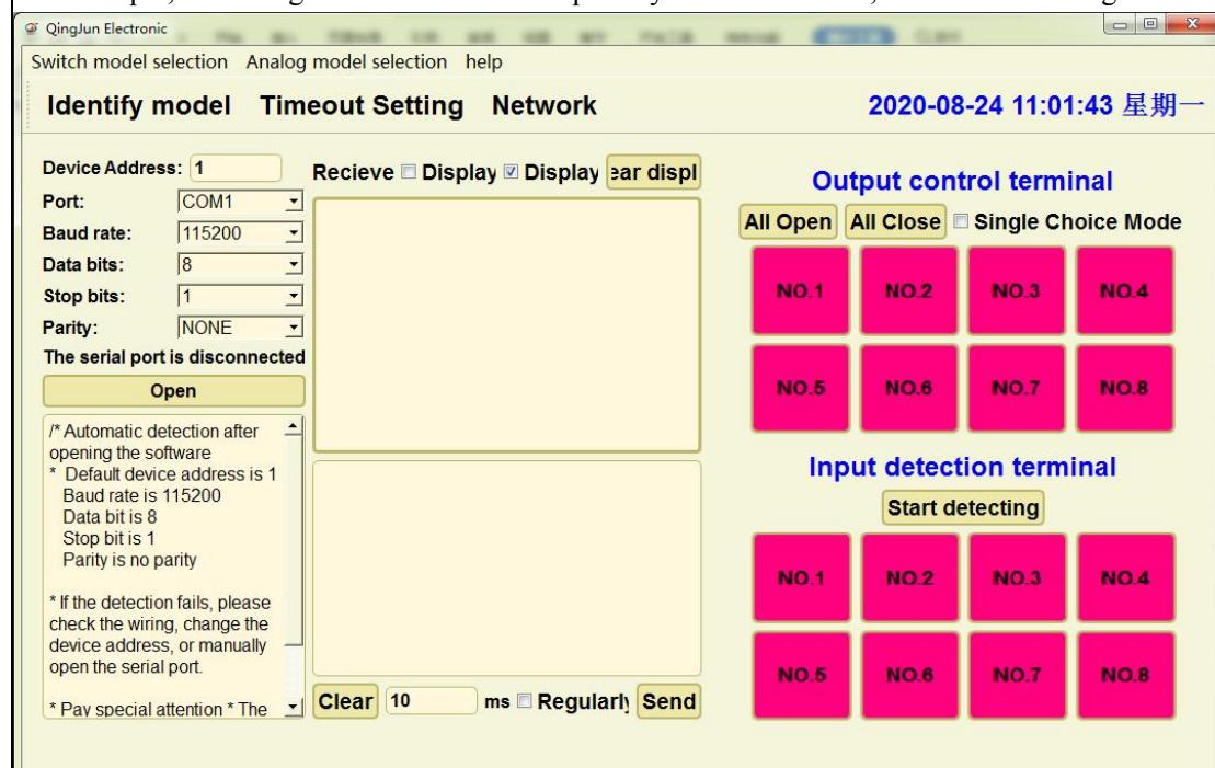
Note: The old-generation products may not be recognized. Don't panic at this time. Manually select the corresponding port and baud rate, click "Open", and then select the corresponding model.
