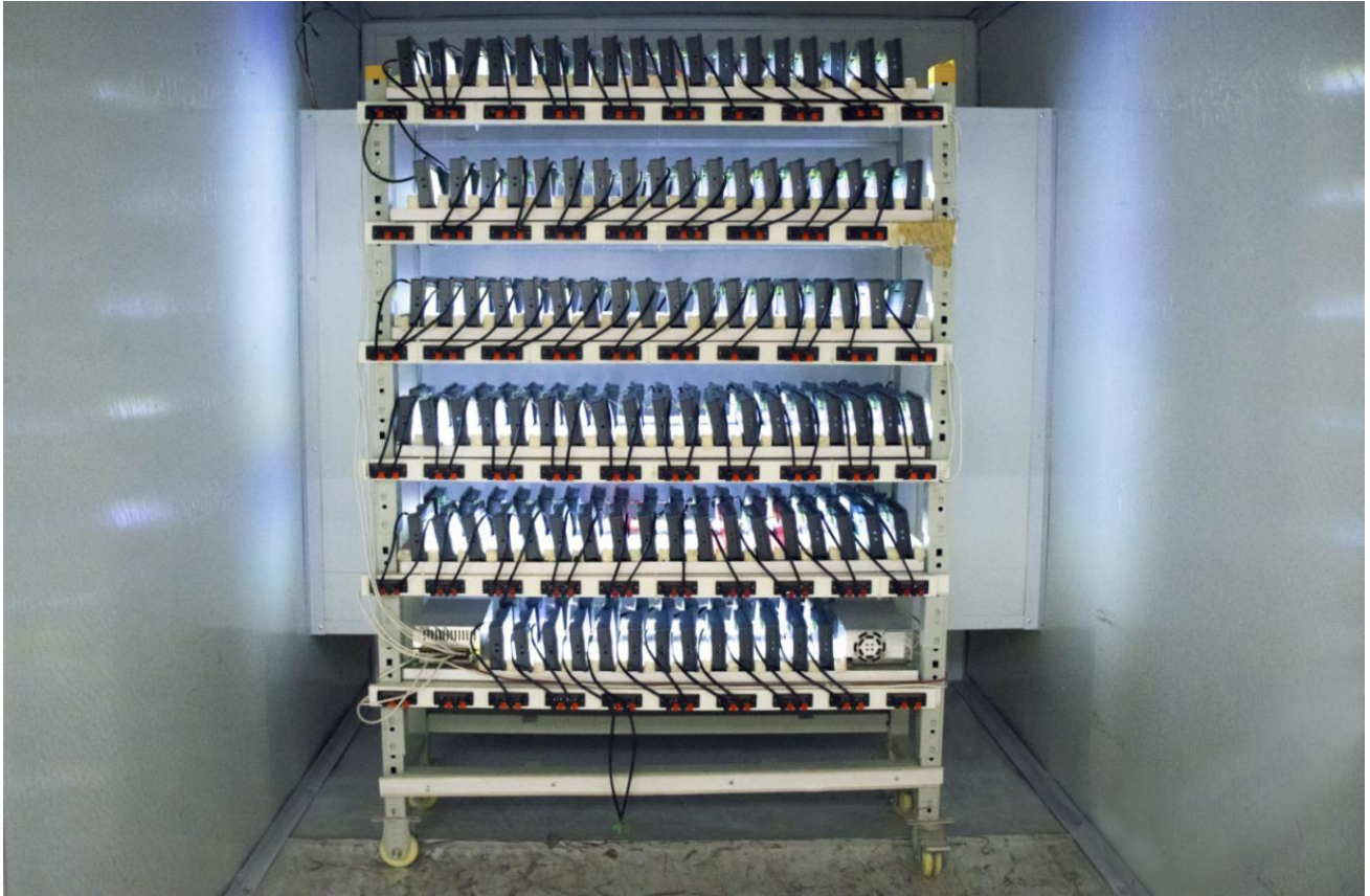
Test Environment: high and low temperature aging test box
