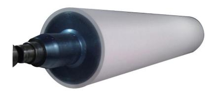
Silicone rollers are usually made of steel or other metals as the roller core, and the surface is wrapped with silicone rubber. Temperature and pressure are strictly controlled during the manufacturing process to ensure the uniformity and durability of the rollers.
