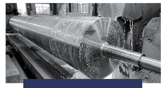
All rollers are precisely calibrated for static balance; for rollers with high design line speeds, dynamic balance calibration is required.
