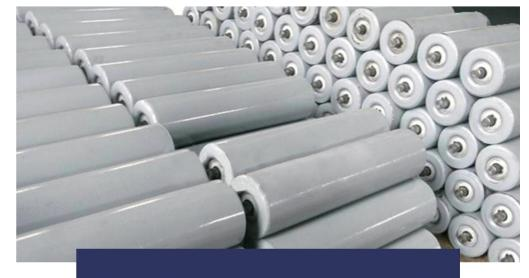
Material: SAE1020, 1045, S355J2H, Q355B, 38CrNiMo, 40Cr, 304L/316L stainless steel, 6063/6061T651 aluminum alloy, etc.
