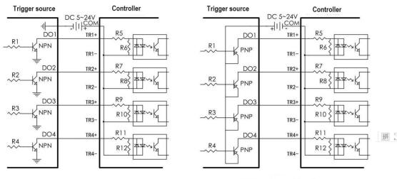
NPN type trigger wiring diagram
