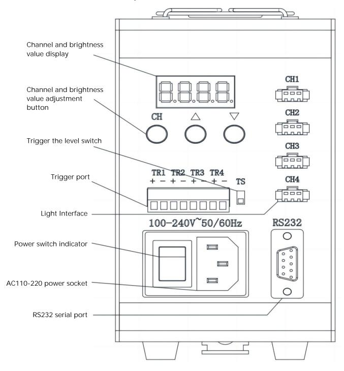
The display adopts a four-in-one digital tube, the first digit indicates the channel number, which can be cut by pressing the "CH" button change the channel number to be set; The last three digits indicate the brightness level of the corresponding channel. The display range is 000-255 (decimal).
