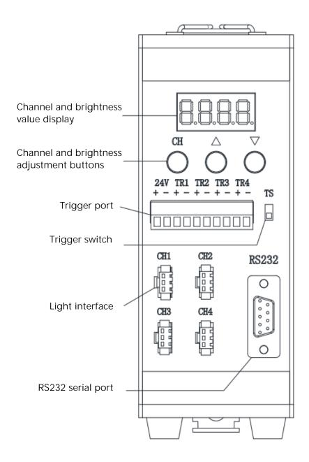
The display adopts a four-in-one digital tube, the first digit indicates the channel number, which can be cut by pressing the "CH" button change the channel number to be set; The last three digits indicate the brightness level of the corresponding channel. The display range is 000-255 (decimal).
