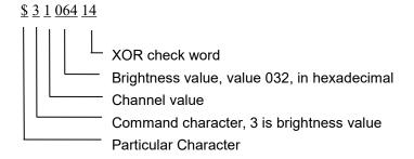
The procedure of the XOR check word algorithm is as follows:
