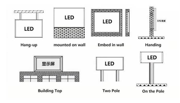
Note: The above are the six installation methods commonly used in the installation of the display screen at present. For the indoor display screen, the four installation methods A\B\C\D are generally adopted, and the above methods can be used for the outdoor display screen.
