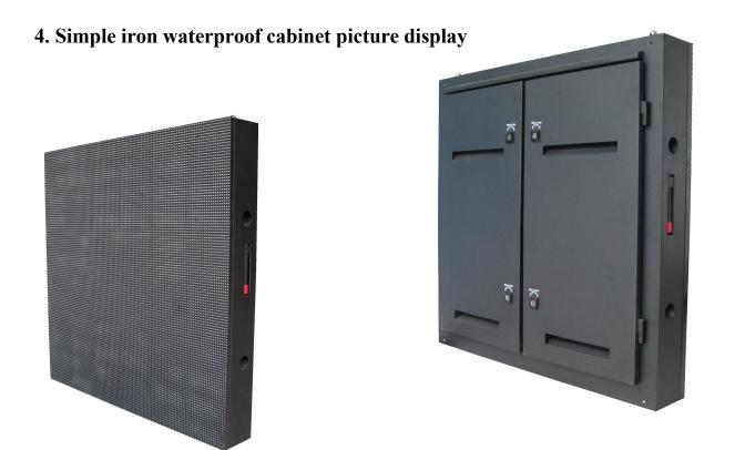
Cabinet features: ·960\*960mm standard iron cabinet, suitable for all 320\*160mm modules. ·Unified installation hole position, unified waterproof rubber ring, unified screw specification, unified power line, interface, unified box specification, unified packaging size, and unified steel structure design.
