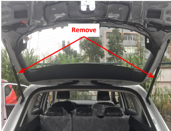
7. Remove the original gas struts.
