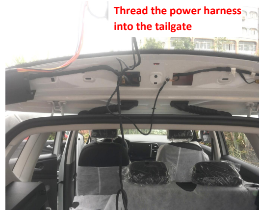
15. Thread the power harness into the tailgate along with original wires.
