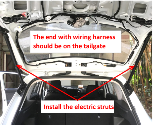
11. Install the electric struts, L on the left and R on the right (the first letter of the strut code).
