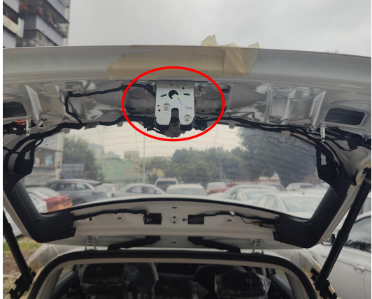
3. Remove the original latch and keep the screws.
