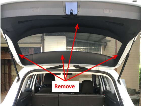
2. Remove the tailgate trim panels.
