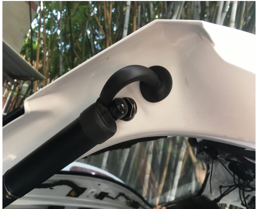
13. Thread the strut wiring harness into the tailgate and plug the hole with the hole plug securely.
