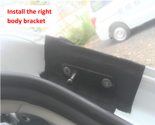
9. Install the right body bracket.
