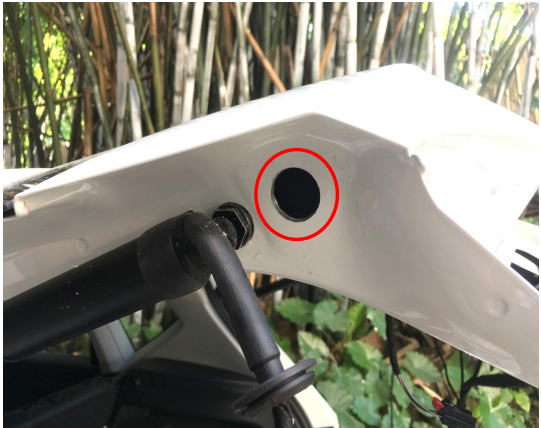
12. Drill a hole at the indicated position on both sides with a 21mm drill bit to allow the wiring harnesses to pass
