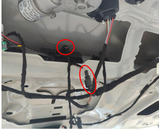
5. Connect the plugs of the lock signal harness to the plugs of original tailgate switch.
