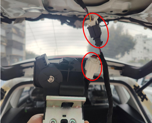
4. Connect the plugs of the lock signal harness to the plugs of the power latch.
