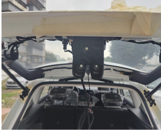
6. Install the power latch (make sure the power latch is in the locked state to prevent from accidental closing).
