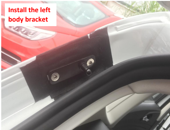
8. Install the left body bracket.
