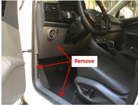
1. Remove the indicated driver side trim panels.
