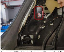
21. Secure the ECU at the indicated position on the left side of the trunk.
