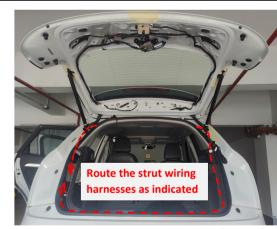
11. Route the strut wiring harnesses to the left side of the trunk as indicated and plug the holes.
