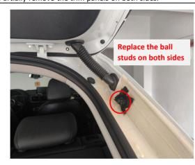
8. Replace the balls stud on both sides of the car body.
