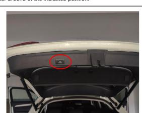
23. Stick the hole template to the indicated position of the trim panel, open a hole and install the added tailgate
