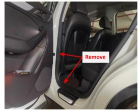
2. Remove the rear left door sill panels and B-pillar trim
