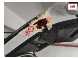
6. Replace the screw in position (1) with our reinforcing ball stud and replace the original ball stud in position (2) with the removed screw.
