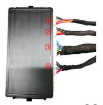
20Insert the left and right strut wiring harnesses ①②, lock signal harness③, and power harness④ into the ECU in sequence.
