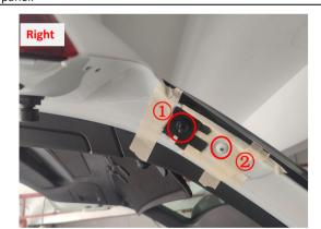
7. Replace the screw in position 1 with our reinforcing ball stud and replace the original ball stud in position 2 with the removed screw.
