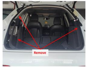
3. Remove the trunk floor mat and the door sill panel. Partially remove the trim panels on both sides.
