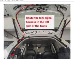
12. Route the lock signal harness to the left side of the trunk along the original wire harness.
