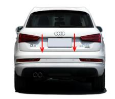
24. Manually close the tailgate to the position where it touches the striker, press the tailgate buttons to open and close the tailgate once to initialize the system and test each function of the electric tailgate.
