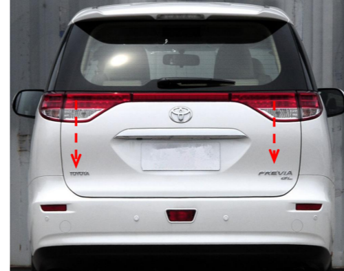
24. Press the added tailgate switch to open and close the tailgate once for initializing the system, and then test each function of the electric tailgate.
