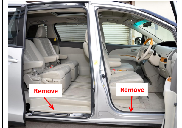
1. Remove the right side door sill panel and step board to allow wiring harnesses to pass through.
