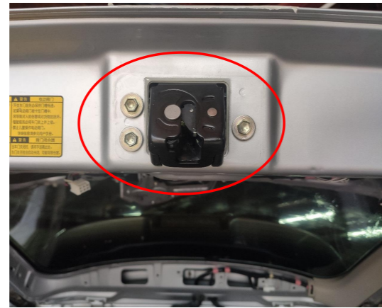
3. Remove the original latch and install our power latch.
