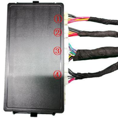
23. Insert the strut wire harnesses ① ②, lock signal harness ③, and power harness ④ into the ECU in sequence, and then mount the ECU onto its bracket.
