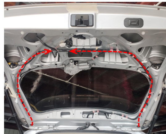
13. Route the strut wiring harnesses.
