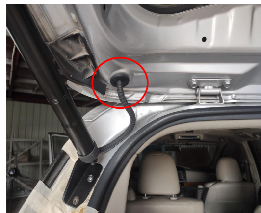
12. Thread the strut wiring harness through the indicated hole into the tailgate.
