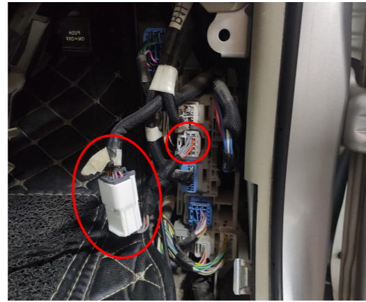
18. Connect the plugs of power harness to the signal plug and its socket.
