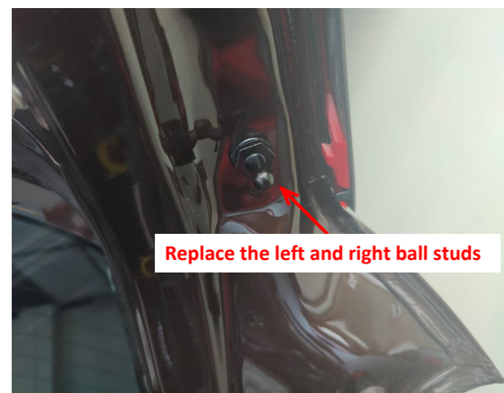
7. Replace the ball studs on both sides with provided ones.
