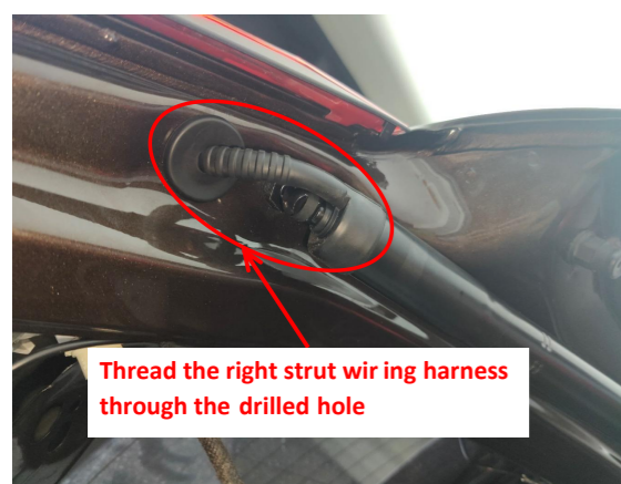
12. Thread the right strut wiring harness into the tailgate through the drilled hole.
