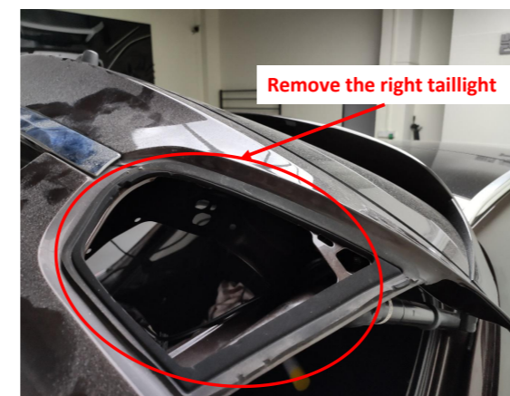
9. Remove the right taillight to avoid damage when drilling hole.
