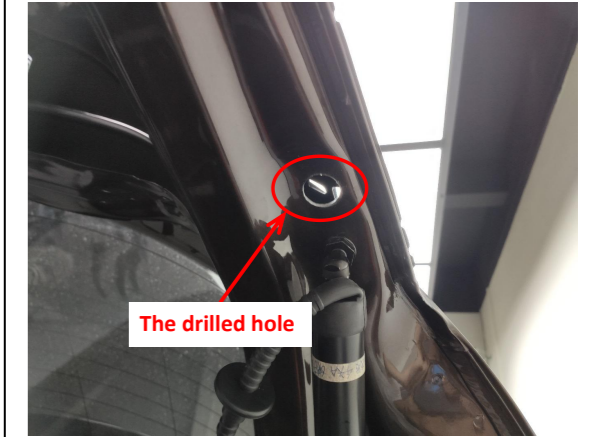
11. Install the taillight back after drilling the hole.
