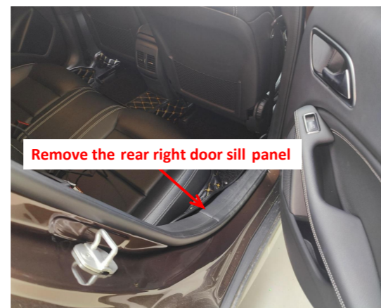
3. Remove the rear right door sill panel to allow the power harness to pass through.
