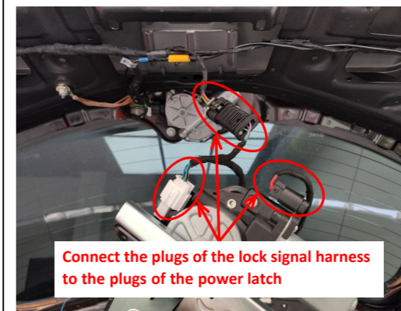
15. Connect the plugs of the lock signal harness to the plugs of the power latch.
