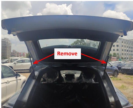
5. Remove the original gas struts.
