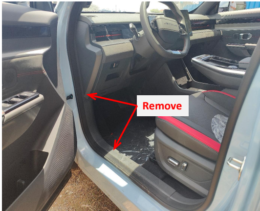
1. Remove the indicated driver side trim panel and door sill panels.
