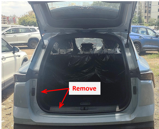
4. Remove the indicated trunk trim panels.
