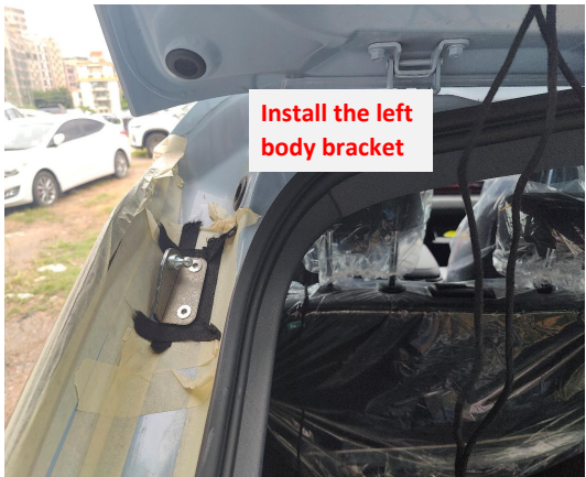
6. Replace the left body bracket and pay attention to the direction.
