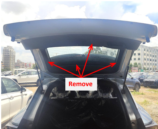
3. Remove the tailgate trim panels.
