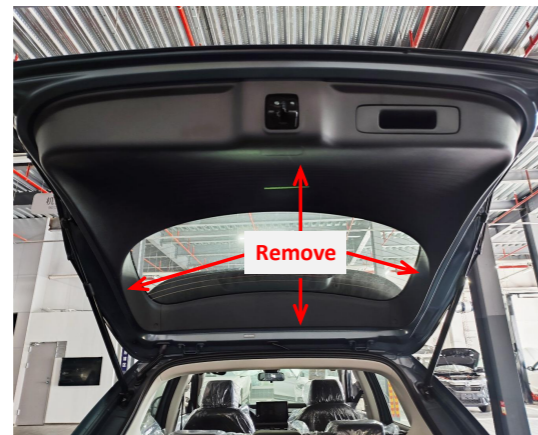
3. Remove the tailgate trim panels.
