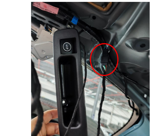
15. Connect the plug of the lock signal harness to the added tailgate switch.
