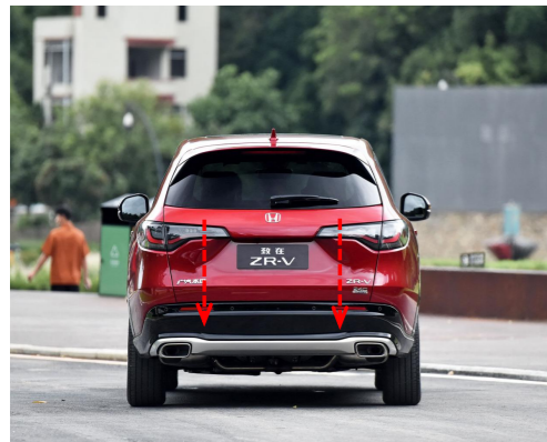
27. Press the added tailgate switch button to open and close the tailgate once, the system completes initialization and then test each function of the electric tailgate.
