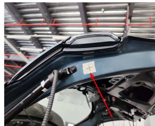
9. Attach the hole template to the indicated location and open a hole to allow the strut wiring harnesses to pass
