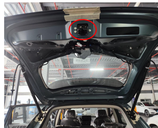
12. Remove the original lock and install our power latch.
