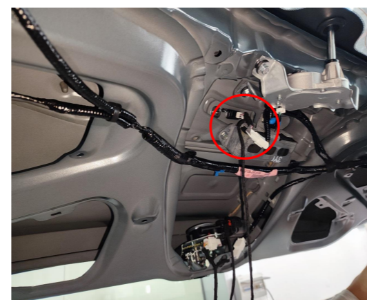
14. Connect the plugs of the lock signal harness to the plugs of the original tailgate switch.
