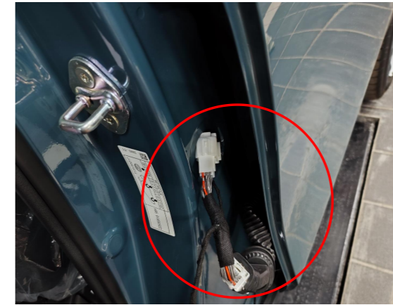
20. Connect the power harness to the B-pillar signal plugs at the rear left side B-pillar.
