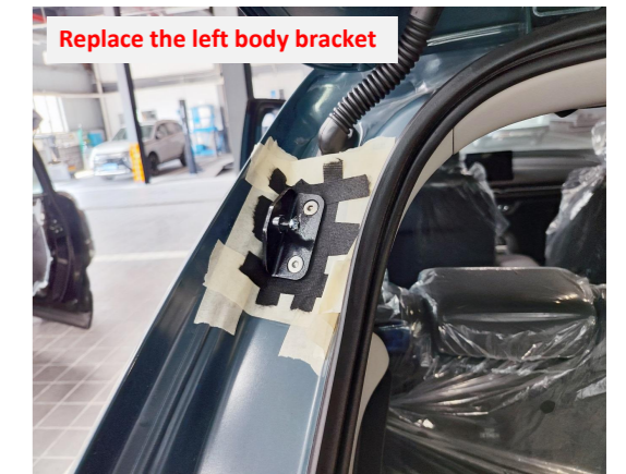
6. Replace the left body bracket.
