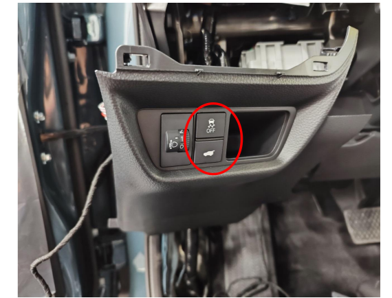
21. Install the added front switch.
