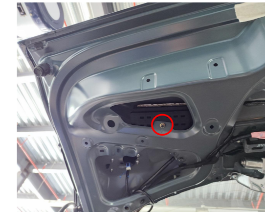
25. Place the ECU bracket at the indicated position and secure it with a nut.
