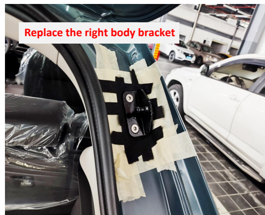
7. Replace the right body bracket
