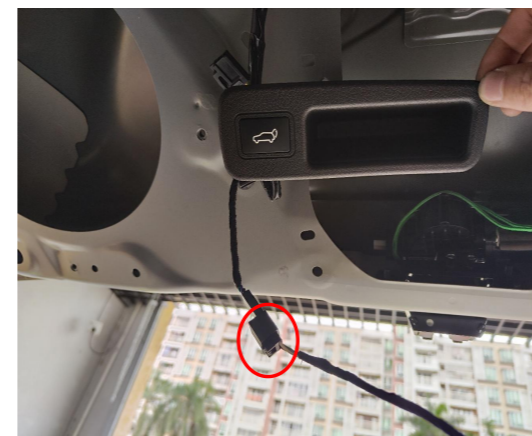
14. Connect the plug of the lock signal harness with the added tailgate switch.
