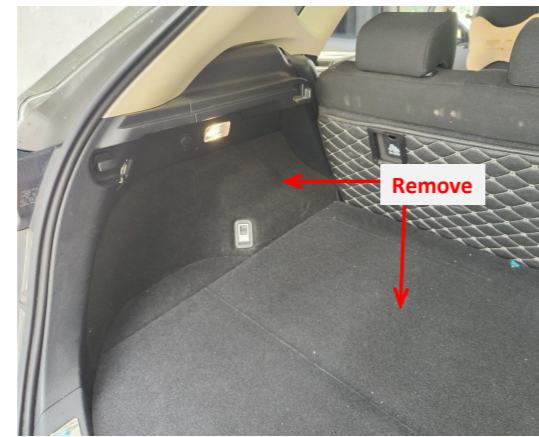
3. Remove the trunk floor mat and the trim panel on the left side.
