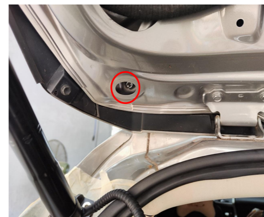
9. Thread the strut wiring harness through the indicated hole into the tailgate; the same on the other side.
