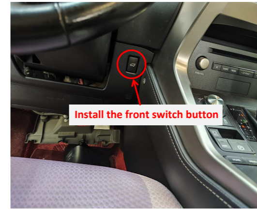
20. Install the front switch button.
