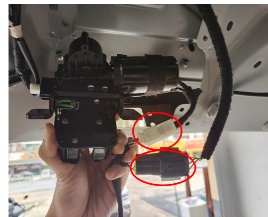
13. Connect the plugs of the lock signal harness with the power latch.
