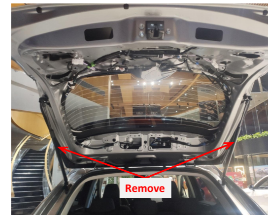
5. Remove the original gas struts.
