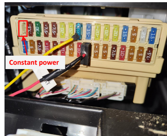
24. The fuse slot for power supply is indicated above.
