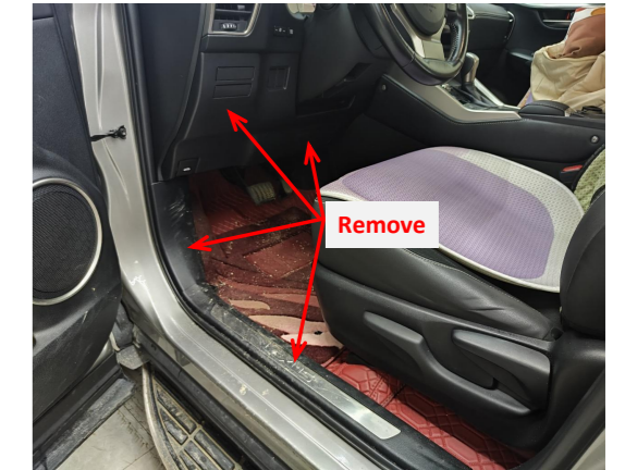
1. Remove the front left door sill panels and switch panel.
