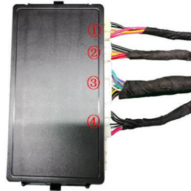
28. Insert the strut wiring harness ①, lock signal harness ②, and power harness ④ into the ECU in sequence.
