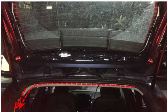
15. Route the strut wiring harnesses as indicated.
