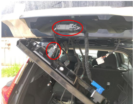
10. Connect the plugs of the lock signal harness to the handle switch.
