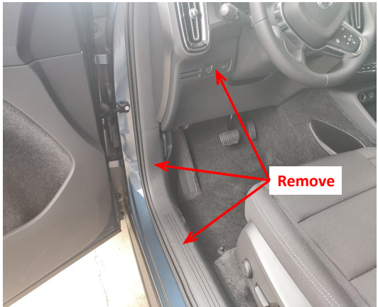
1. Remove the front left side door sill panels and the switch panel.
