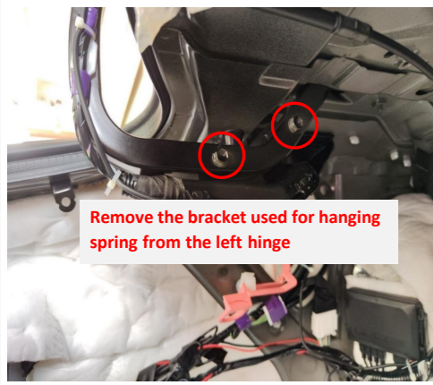
9. Remove the bracket used for hanging spring from the left hinge.
