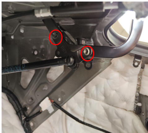
10. Remove the bracket used for hanging spring from the right hinge.
