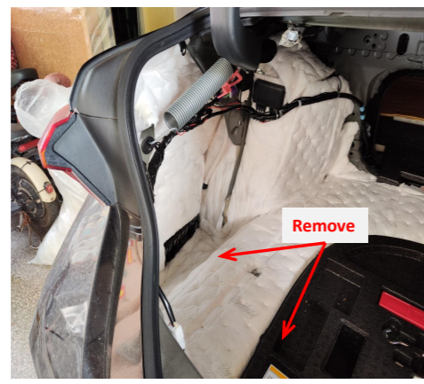
4. Take out the trunk floor mat and remove the trim panel on both sides of the trunk.
