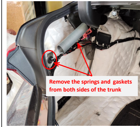
7. Remove the springs and gaskets from both sides of the trunk.
