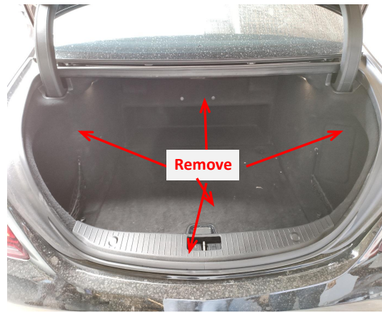
2. Remove the indicated trim panels from the trunk.
