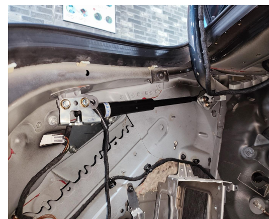
12. Install the left electric strut (the first letter of the strut code shows the L/R).
