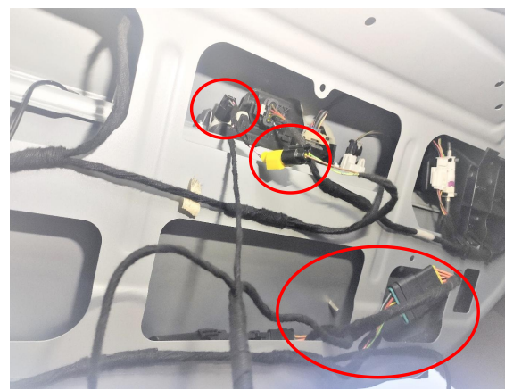
17. Connect the plugs of the lock&power harness to the original tailgate switch.
