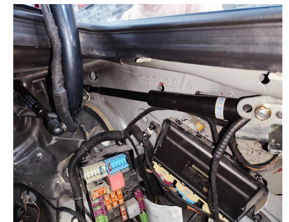
11. Install the right electric strut (the first letter of the strut code shows the L/R).
