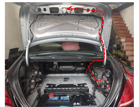
21. Route the power harness as indicated (routing only, no plug or power connection).
