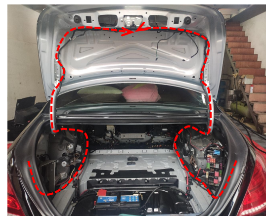
20. Route the strut wiring harnesses as indicated.
