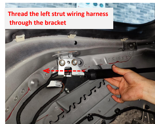
13. Thread the left strut wiring harness through the left bracket.
