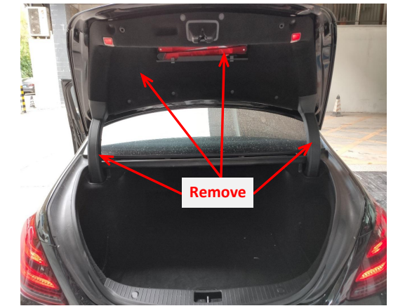
1. Remove the trim panels of the tailgate and hinges.
