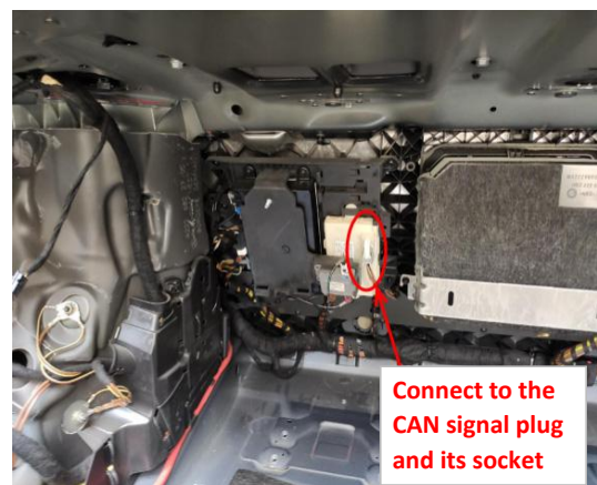
19. Unplug the plug on the left side of the trunk and connect the plugs of the lock&power harness to it and its socket.
