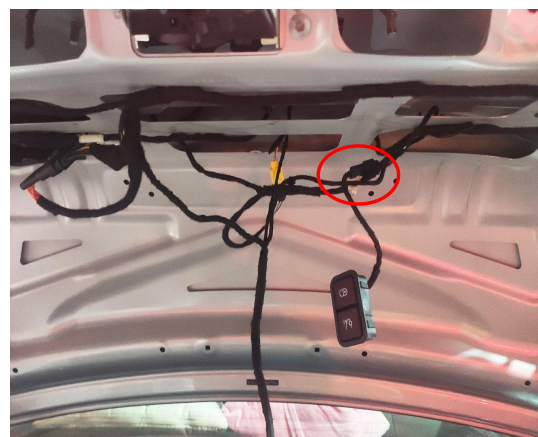
18. Connect the plug of the lock&power harness to the added tailgate switch.
