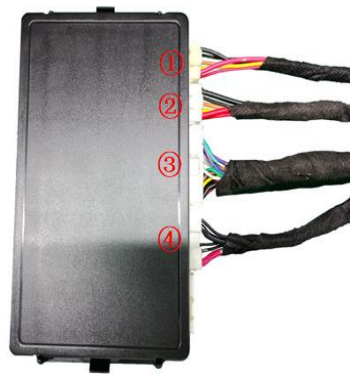
27. Insert the strut wire harness ①, lock signal harness ②, and power harness ④ into the ECU in sequence.
