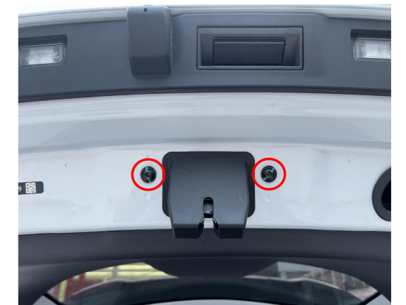
11. Remove the plastic casing of the latch and remove the latch.
