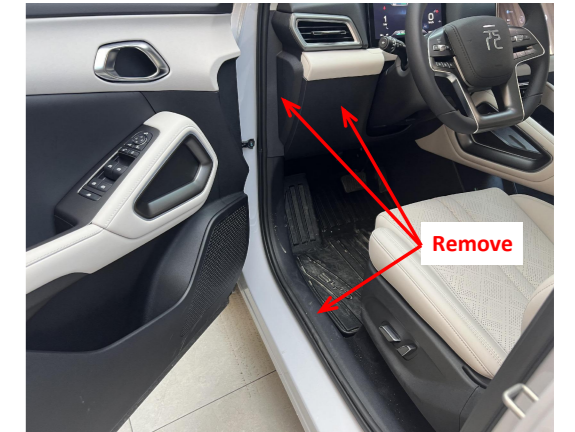
1. Remove the front left door sill panel and the trim panels of the fuse box.
