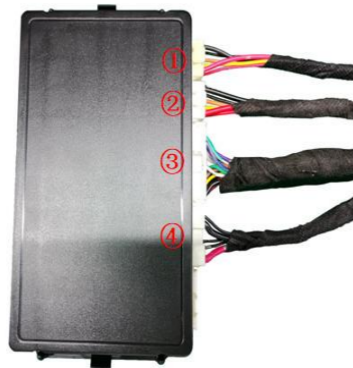
23. Insert the left and right strut wiring harnesses ① ②, lock signal harness ③, and power harness ④ into the ECU in sequence.
