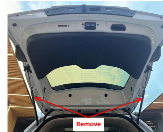
5. Remove the original gas struts.
