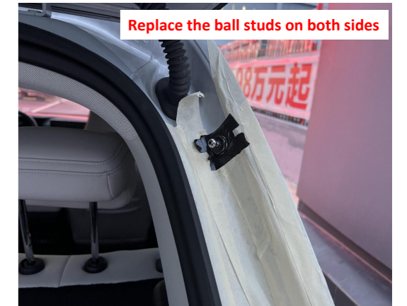
6. Replace the ball studs on both sides.
