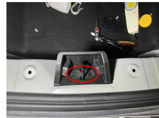
25. If the tailgate doesn't close properly, you can adjust the position of the lock striker.
