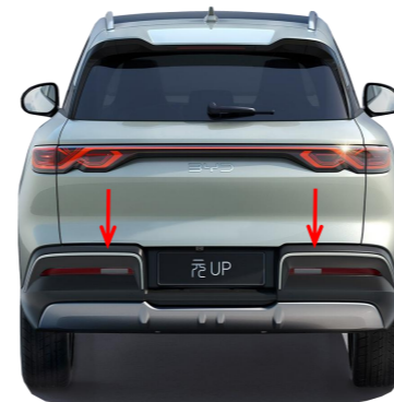
24. Press the added tailgate switch button to close the tailgate once to complete initialization and then test each function of the electric tailgate.
