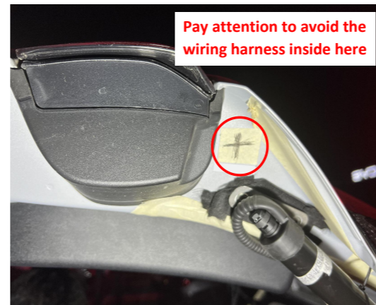
9. Drill a hole at the indicated position on both sides with a \phi 21mm drill bit to allow strut wiring harness to pass through.
