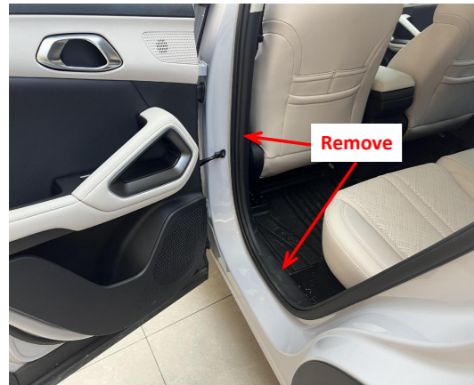
2. Remove the rear left door sill panel and the B-pillar trim panel.
