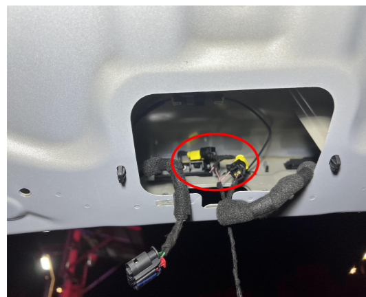
12. Connect the plugs of the lock signal harness to the original tailgate switch.
