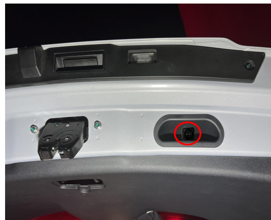
27. Install the added tailgate switch and reinstall all the trim panels.
