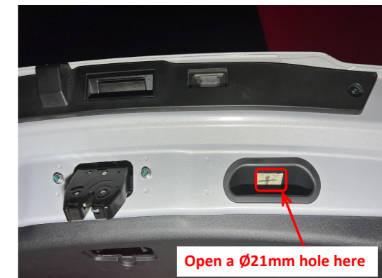
26. Remove the tailgate handle and open a Ø21mm hole with the provided hole opener for installing the added tailgate switch.
