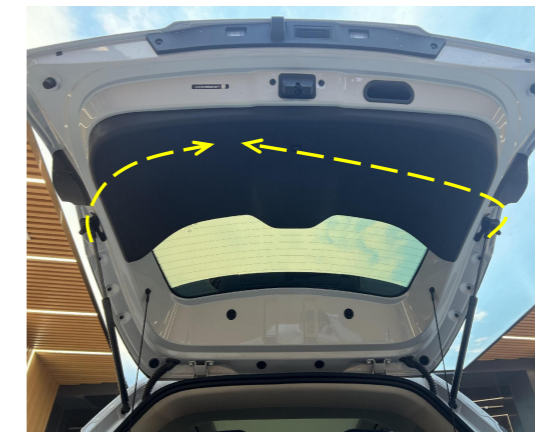
10. Thread the left and right strut wiring harnesses to the indicated position.
