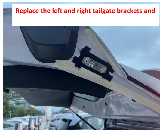
7. Replace the left and right tailgate brackets.
