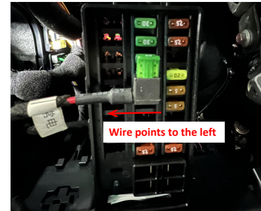
20. Plug the fuse tap into the fuse box and pay attention to the direction of wire.
