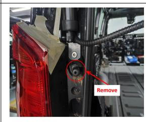
11.Remove the indicated bump stops on both sides.
