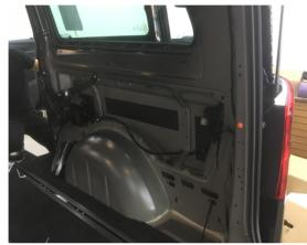
3. Remove the trim panel on the right side of the trunk to allow the strut wiring harnesses to pass through.
