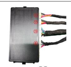
26. Insert the strut wiring harnesses (1)(2), lock signal harness (3), and power harness (4) into the ECU in sequence and then fit the ECU onto its bracket.
