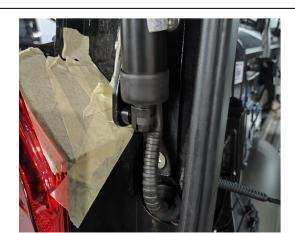
12. Thread the strut wiring harness into the car body and plug the hole securely.
