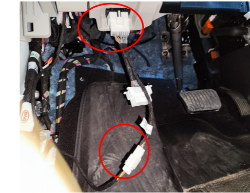
24. Remove the OBD plug from its slot, connect power harness to it, hide the pair of plugs behind the panel and place our OBD plug in the slot of original OBD plug.
