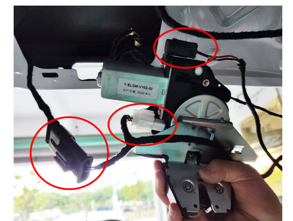
16. Connect the the plugs of lock signal harness to our power latch.
