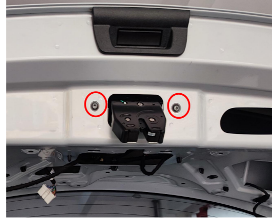
18. Install the power latch and fasten it with provided screws.
