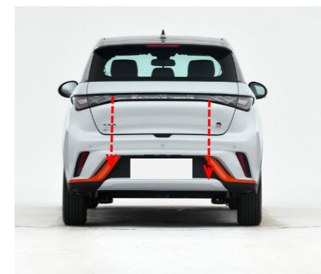
30. Press the added tailgate switch to open and close the tailgate once for initializing the system, and then test the functions of the electric tailgate.
