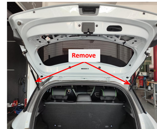
5. Remove the original gas struts.
