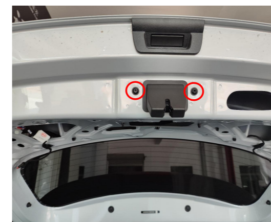
15. Remove the original latch.
