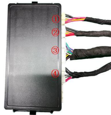
29. Insert the strut wiring harnesses ①②, lock signal harness ③, and power harness ④ into the ECU in sequence.
