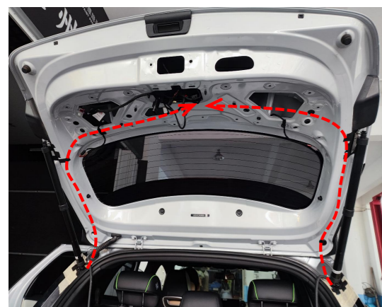
12. Route the strut wiring harnesses to the tailgate.
