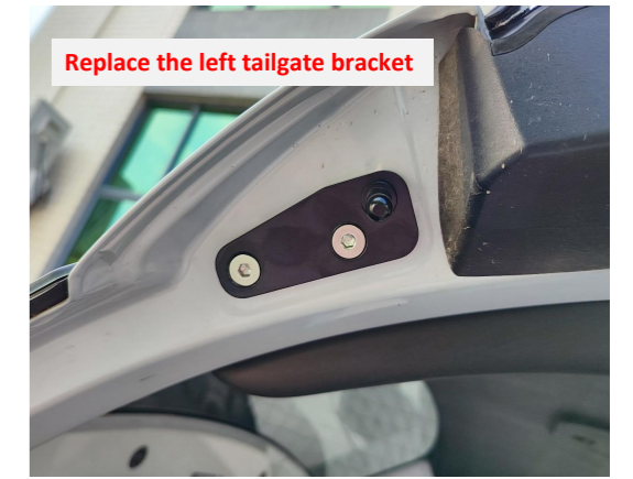
6. Replace the left tailgate bracket with provided one.
