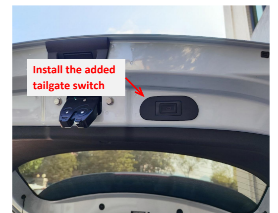
31. Reinstall all trim panels and install the added tailgate switch.
