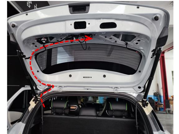
21. Route the power harness to the tailgate.
