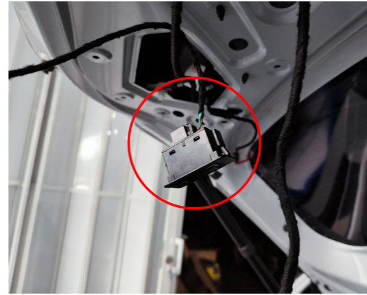
19. Connect the lock signal harness to the plug of added tailgate switch.
