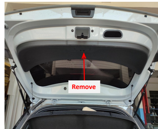
3. Remove the tailgate trim panel.
