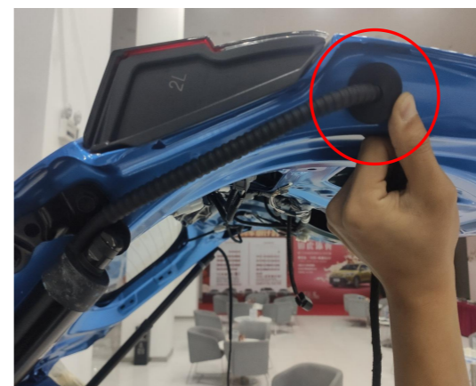
10. Thread the strut wiring harnesses through the holes on both sides into the tailgate and plug the holes securely.
