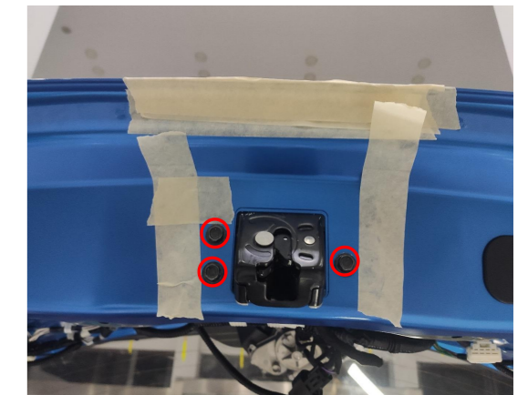
11. Replace the original latch with our power latch.
