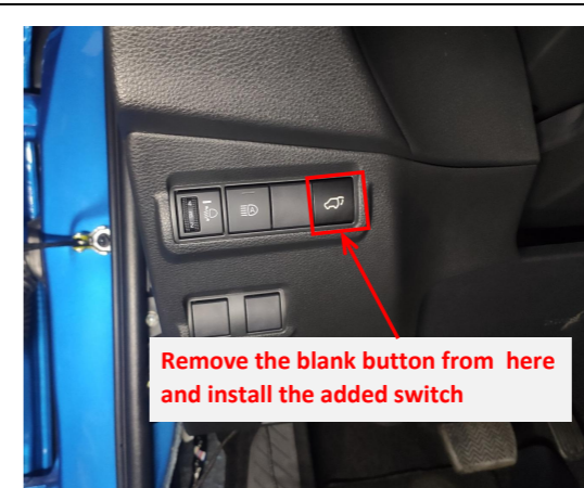
20. Remove the blank button, install the added front switch and connect the plugs behind the switch panel for backlight.
