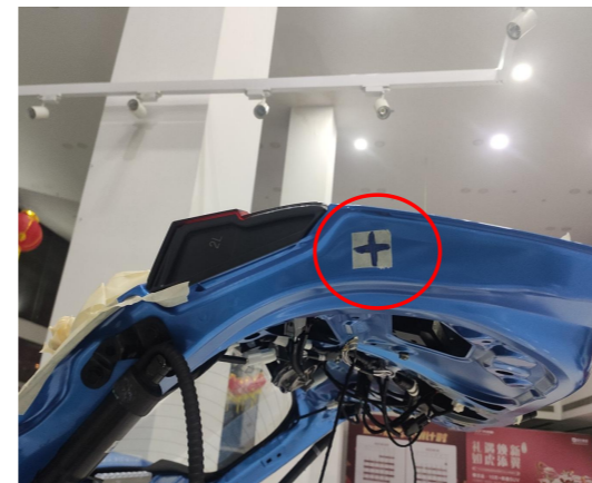
9. Drill a hole at the indicated position with a \phi 21\text{mm} drill bit to allow the strut wiring harnesses to pass through.
