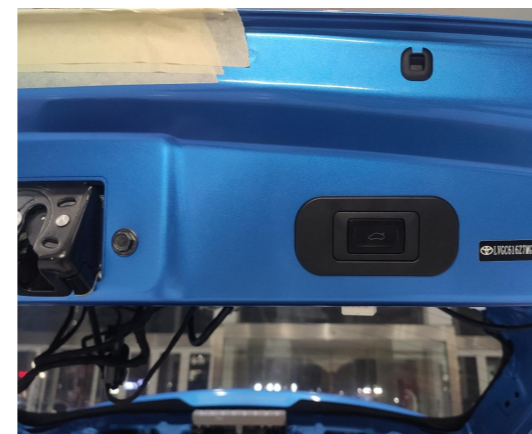
14. Connect the plug of the lock signal harness to the added tailgate switch.
