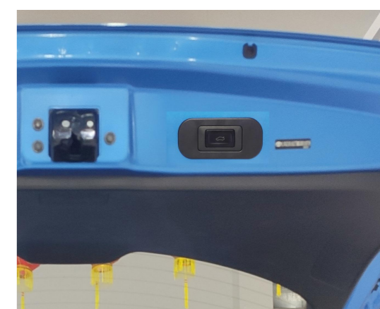
26. Reinstall all trim panels and install the added tailgate switch.
