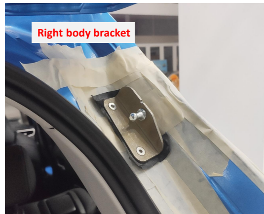
7. Replace the bracket on the right side of the car body.
