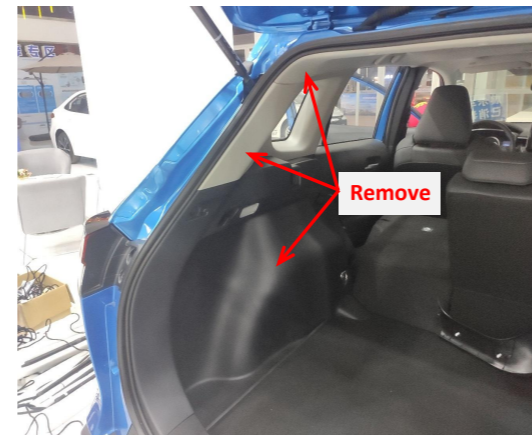
4. Remove the trim panels on the left side of the trunk.
