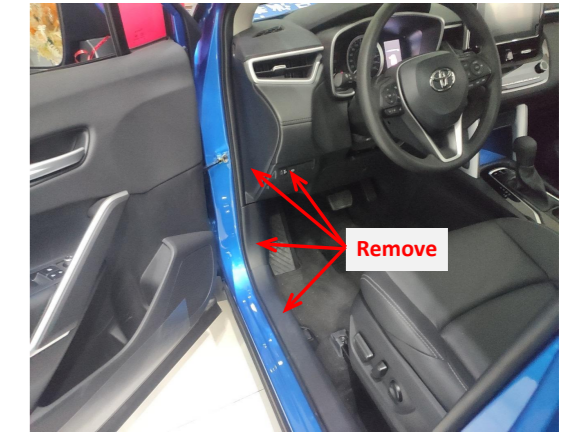
1. Remove the front left side trim panel, door sill panel and switch panel.
