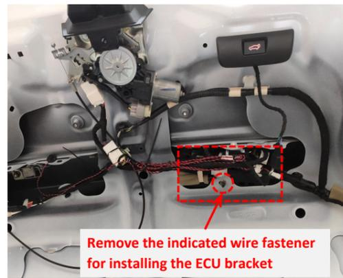
18. Install the ECU bracket at the the indicated position and secure it with a nut.
