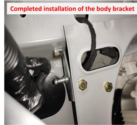
4. The completed installation of the body bracket. Both sides are the same.
