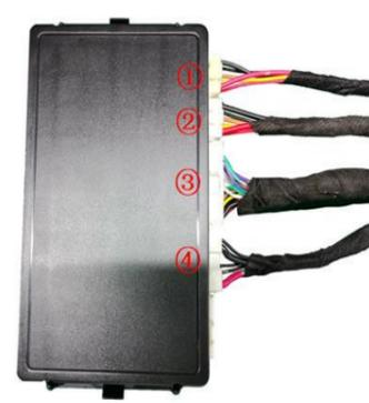
19. Insert the left and right strut wiring harnesses ①②, lock signal harness ③, and power harness ④ into the ECU in sequence.
