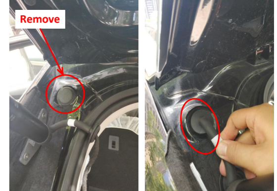
11. Remove the rubber plug to allow the strut wire harness to pass through and then plug the hole tightly; both sides are the same.
