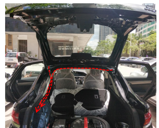
12. Route the strut wire harnesses.
