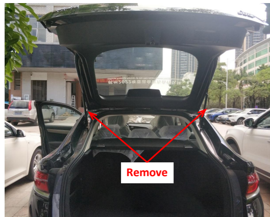
7. Remove the original gas struts.
