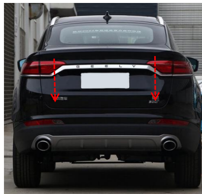
27. Press the added tailgate switch button to open and close the tailgate once for initializing the system, and then test the functions of the electric tailgate.
