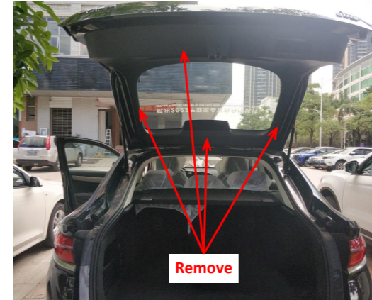
5. Remove the tailgate trim panels.
