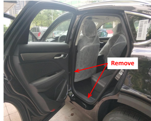
4. Remove the rear left side door sill panel and B-pillar trim panel.
