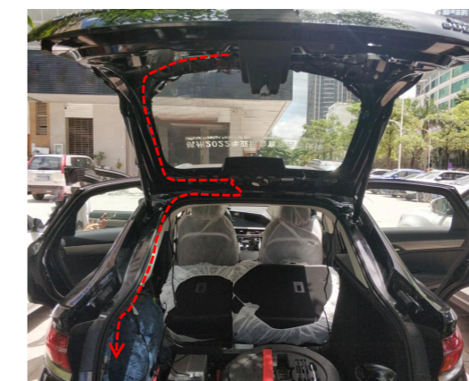
15. Route the lock signal harness to the left side of the trunk.
