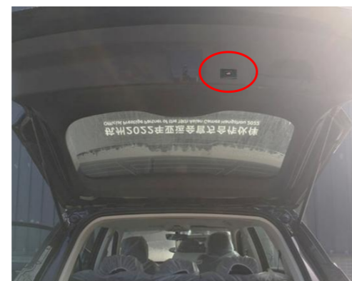
28. Install all trim panels back and install the added tailgate switch (remove the small cover panel).
