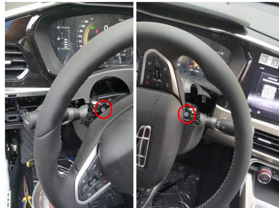
2. Remove the steering wheel trim panels (there are screws in the circles).
