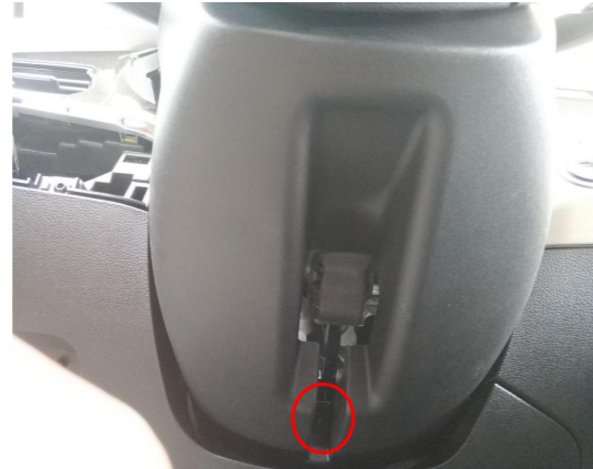
3. Remove the steering wheel trim panels (there are screws in the circles).
