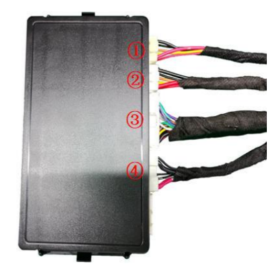
26. Insert the strut wire harnesses ① ②, lock signal harness ③, and power harness ④ into the ECU in sequence and then mount the ECU onto its bracket.
