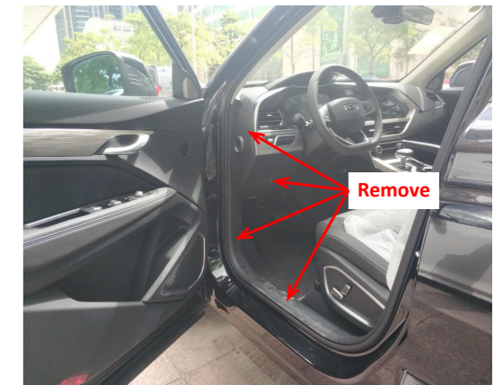
1. Remove the front left side trim panels, door sill panel and storage box.
