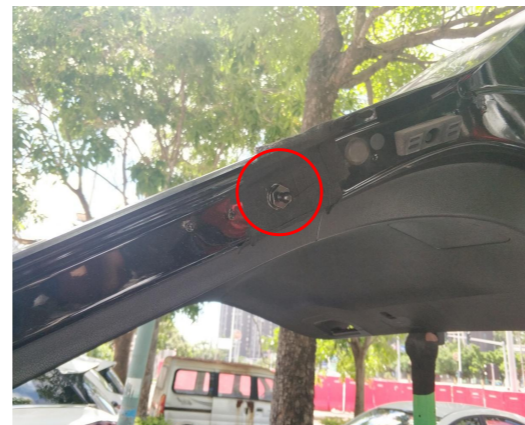
9. Replace the tailgate ball studs.
