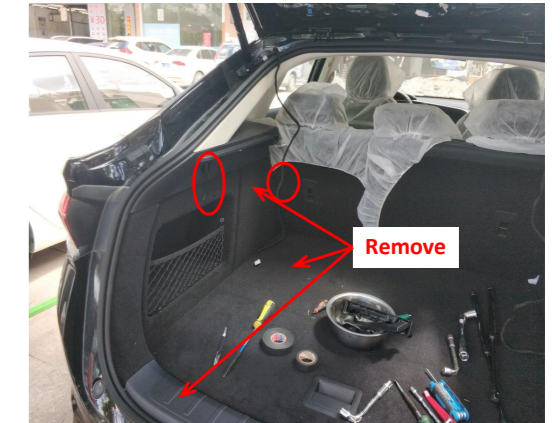
6. Remove the trunk floor mat, door sill panel and the trim panels on the left side (there are screws in the circles).
