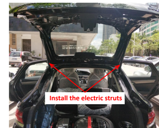
10. Install the electric struts, L on the left and R on the right (the first letter of the strut number).
