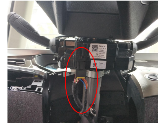
21. Connect the power harness with the signal plug and its socket under the steering wheel.
