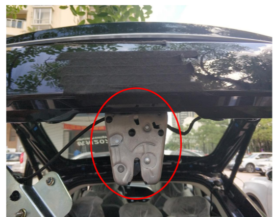
13. Replace the original lock with our lock latch.
