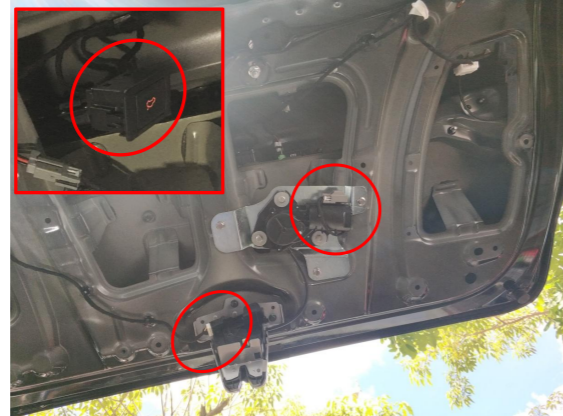
18. Connect the lock signal harness with the plugs of the lock latch, actuator and the added tailgate switch.
