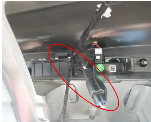
17. Connect the lock signal harness with the plugs of the original tailgate switch.
