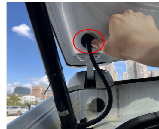
10. Thread the strut wiring harness into the tailgate through the indicated hole.
