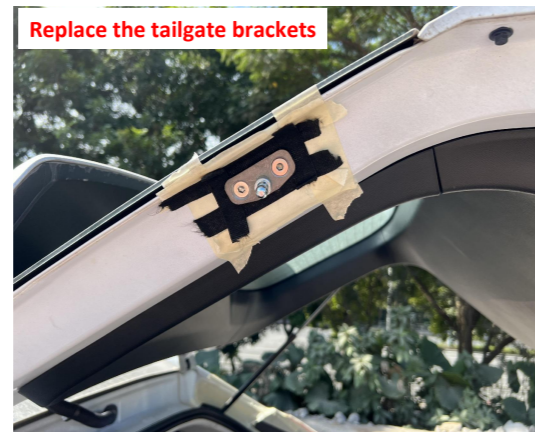
8. Replace the brackets on the tailgate with the ball stud on the lower side.
