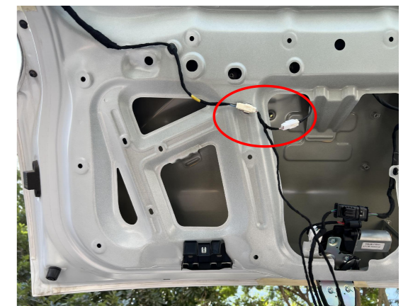
16. Connect the lock signal harness to the plugs of original tailgate switch.
