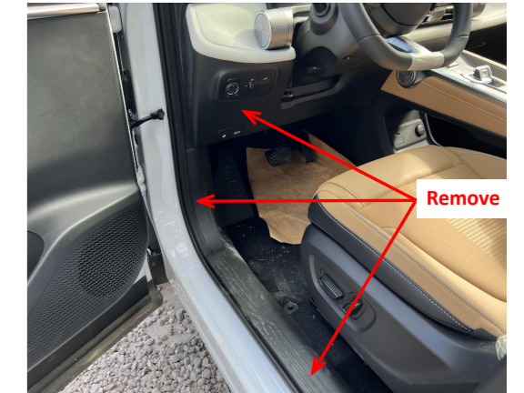
1. Remove the front left side door sill panels and storage box.
