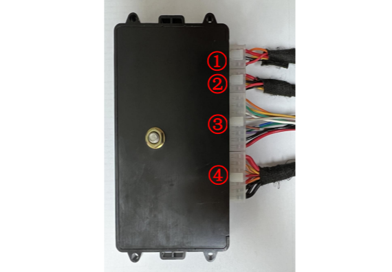
24. Insert the left and right strut wiring harnesses ①②, lock signal harness ③, and power harness ④ into the ECU in sequence.
