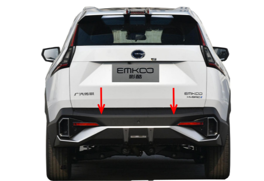
25. Press the added tailgate switch button to close the tailgate once for initializing the system, then test each function of the electric tailgate.
