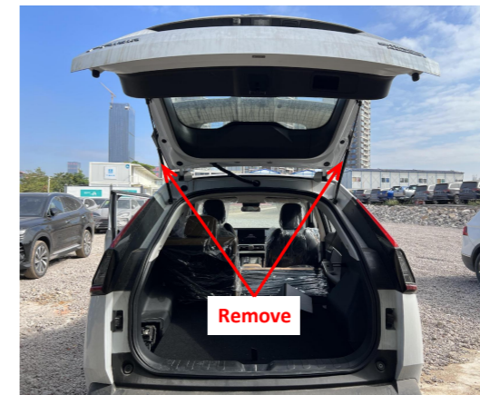
5. Remove the original gas struts.
