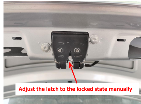
18. Install the lock actuator and secure it with original screws. Manually adjust the latch to the locked state to prevent accidental closing during the installation
