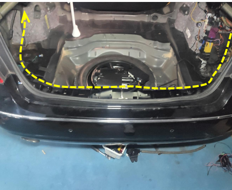
15. Route the right strut harness to the left side of the trunk and tie it along with the original wiring harness.
