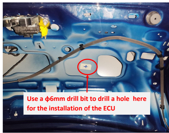
28. Use a \phi 6\text{mm} drill bit to drill a hole at the indicated position for the the installation of the ECU.
