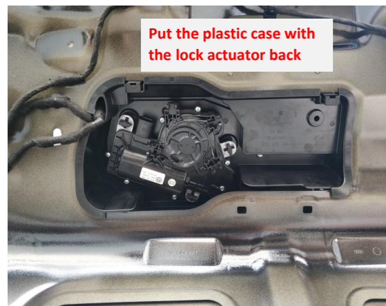
17. Put the plastic housing and the lock actuator back.
