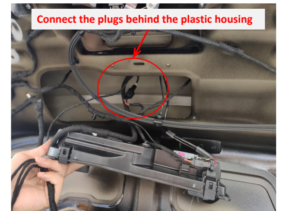
16. Connect the plugs of the lock signal harness to the original tailgate switch.
