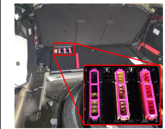
26. Connect to the fuse box for power supply (all the vacant slots are constant power).
