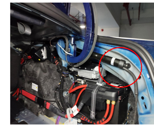
10. Install the right electric strut at the position of the original gas strut, and pay attention to the direction.
