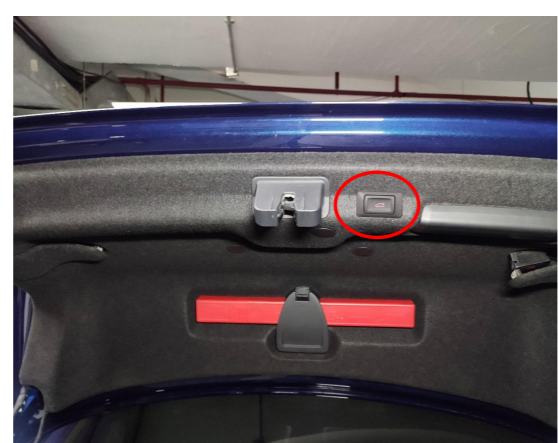
33. Reinstall all the trim panels and fit the added switch in.
