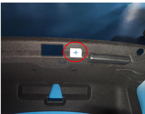
32. Stick the hole template to the indicated position of the tailgate.
