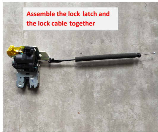
18. Assemble the lock latch and the cable together.
