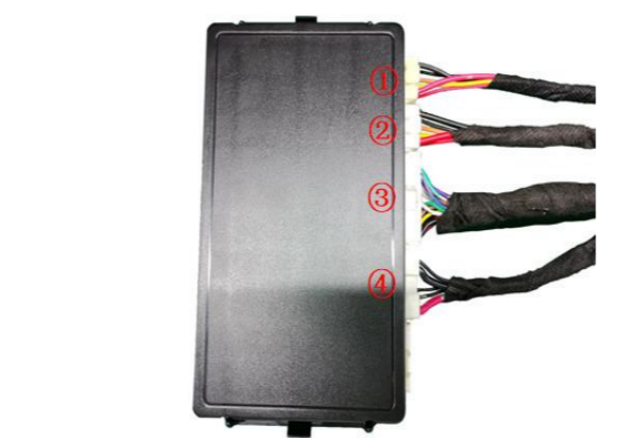
29. Insert the strut wiring harnesses ①②, lock signal harness ③, and power harness ④ into the ECU in sequence and mount the ECU onto its bracket.
