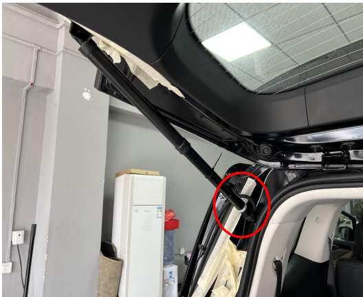
7. Install the electric struts, L on the left and R on the right (the first letter of the strut code).
