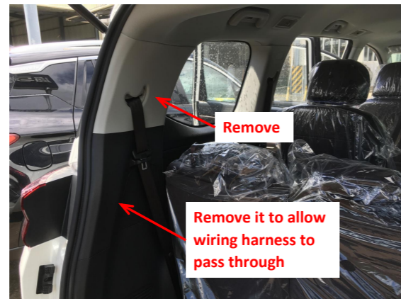
3. Remove the indicated trim panels on the left side of the trunk.
