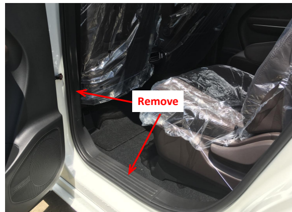
2. Remove the rear left door sill panel and B-pillar trim panel.
