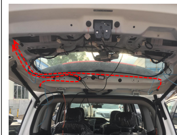
15. Route the strut wiring harnesses as indicated.
