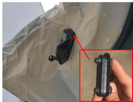
12. Add a shim to the brackets on both sides of the tailgate and replace the bolts with our long bolts.
