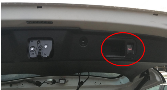
27. Install the added tailgate switch and reinstall all the trim panels.
