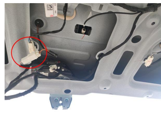
8. Connect the plugs of the lock signal harness to the plugs of original tailgate switch and added tailgate switch.
