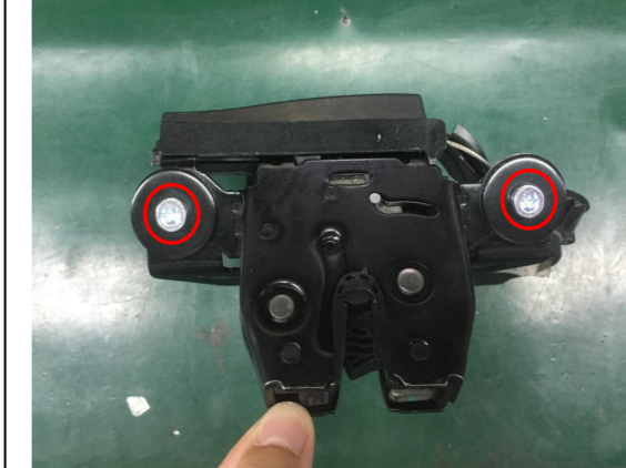
5. Remove the indicated screws from the power latch (keep the shims).
