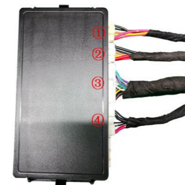
25. Insert the left and right strut wiring harnesses ①②, lock signal harness ③, and power harness ④ into the ECU in sequence.
