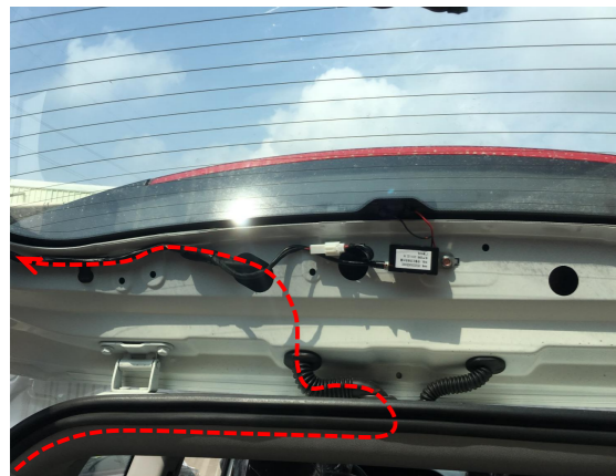
17. Thread the power harness through the tube into the tailgate.
