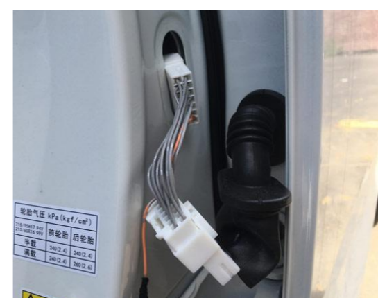
20. Connect to the B-pillar plugs at the rear left B-pillar.
