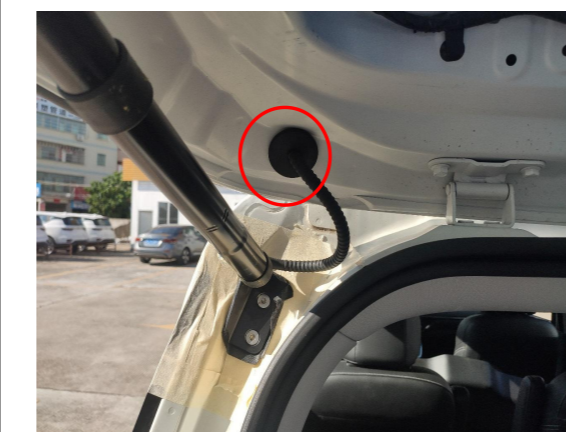
14. Thread the strut wiring harness through the indicated hole into the tailgate.
