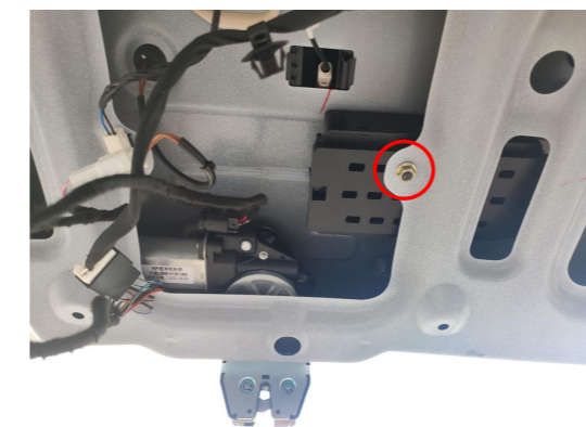
24. Secure the ECU at the indicated position (remove the original cable clip).
