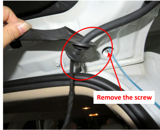
18. Remove the screw from the hole and thread the strut wiring harness through the hole.
