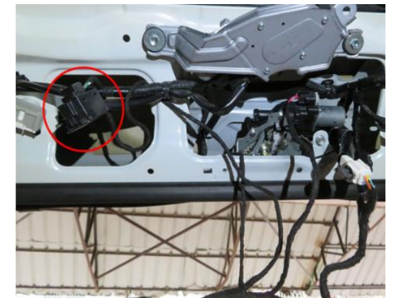
11. Connect the plug of the lock signal harness to the added tailgate switch.
