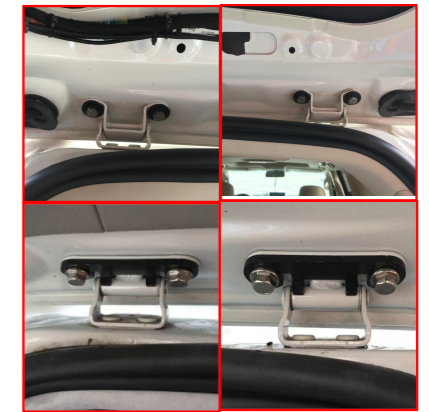
1. Install the corresponding reinforcing washers to the hinges with provided screws according to different vehicle models.
