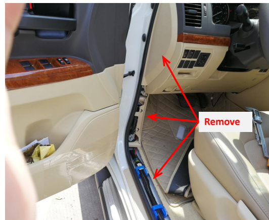
2. Remove the front left side trim panels, door sill panel and storage box.
