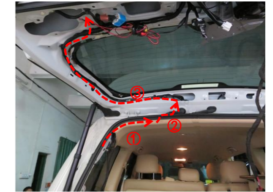
21. Thread the power harness to the left side of tailgate (do not connect plugs before inserting terminals into wiring harness connector).
