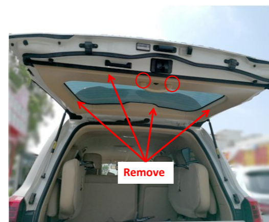
4. Remove the tailgate trim panels (there are screws in the circles).
