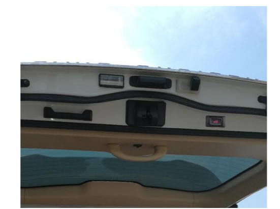
33. Reinstall all the trim panels and install the added tailgate switch.
