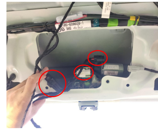
10. Connect the plugs of the lock signal harness to the power latch.
