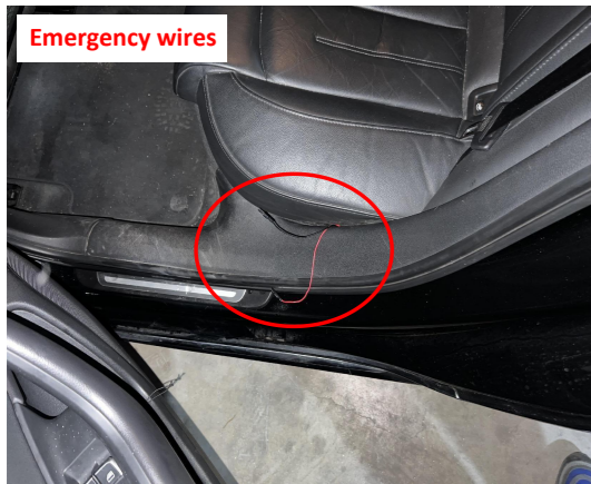
22. Hide the emergency wires under the rear left door sill panel.
