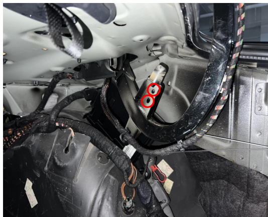
7. The two hole under the bump stop are for the installation of the tailgate bracket.
