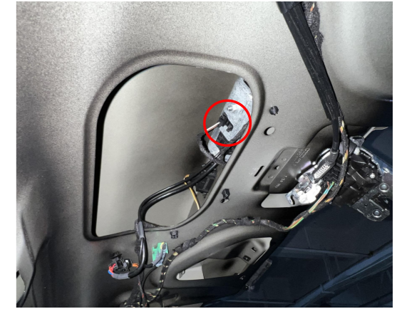
21. Connect the plugs of the lock signal harness to the plugs of original tailgate switch and reinstall the cover.
