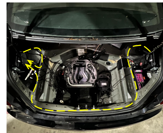
14. Route the strut wiring harness along with original wires to the left side of the trunk.
