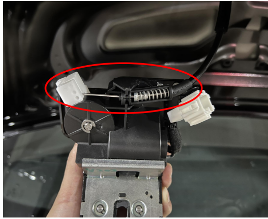
17. Fit the emergency cable onto the power latch.
