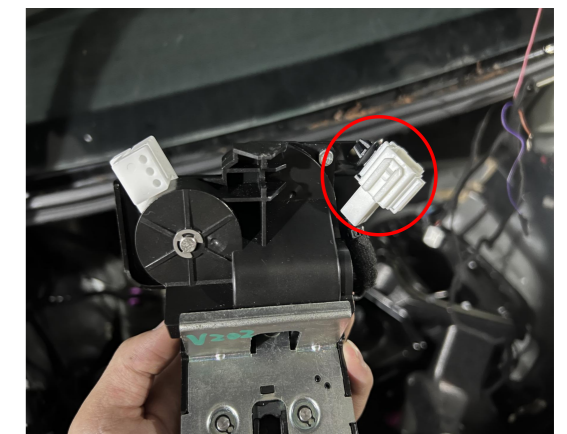
16. Remove the indicated female connector from the power latch.
