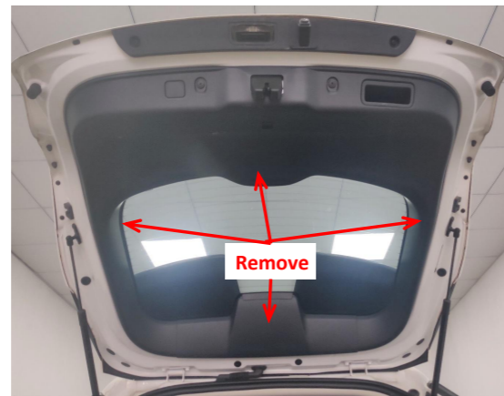
3. Remove the tailgate trim panels.
