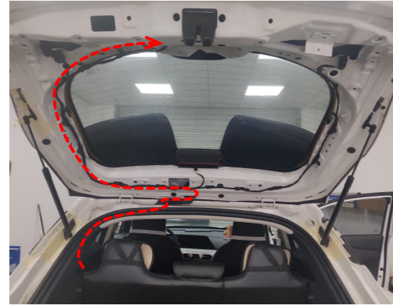
18. Route the power harness to the tailgate (Routing only, no plug or power connection).
