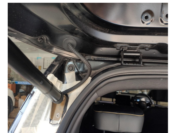
13. Leave a certain length of tube outside to prevent strut wiring harness from being bent, the same on both sides.
