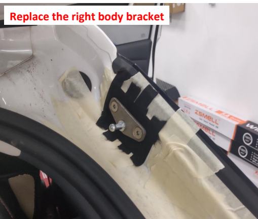
7. Replace the right body bracket.
