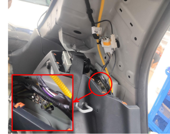
20. Ground at the indicated location (behind the left rear seat).
