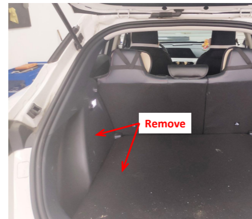
4. Take out the trunk floor mat and foam storage box. Remove the trim panel on the left side of the trunk.
