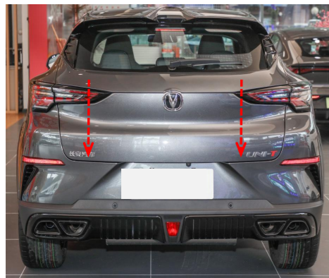
27. Press the added tailgate switch button to open and close the tailgate once, the system completes initialization, and then test each function of the electric tailgate.
