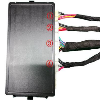
26. Insert the strut wiring harnesses ①②, lock signal harness ③, and power harness ④ into the ECU in
