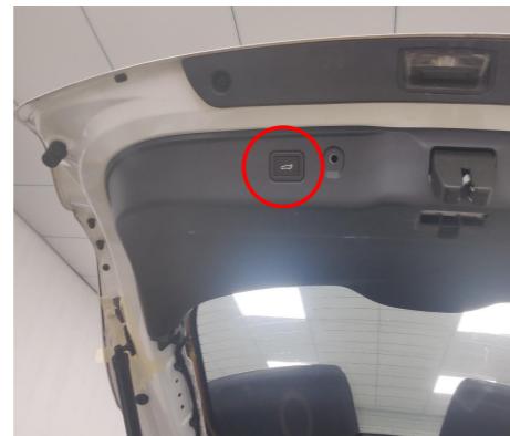
28. Reinstall all trim panels and install the added tailgate switch.
