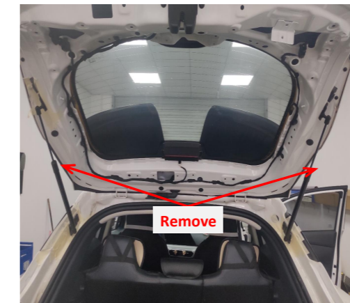
5. Remove the original gas struts.
