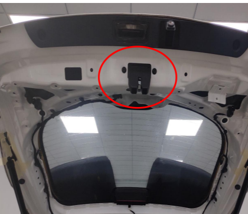
14. Remove the original latch and install our power latch.
