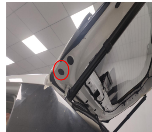
9. Thread the strut wiring harness through the indicated hole into the tailgate.
