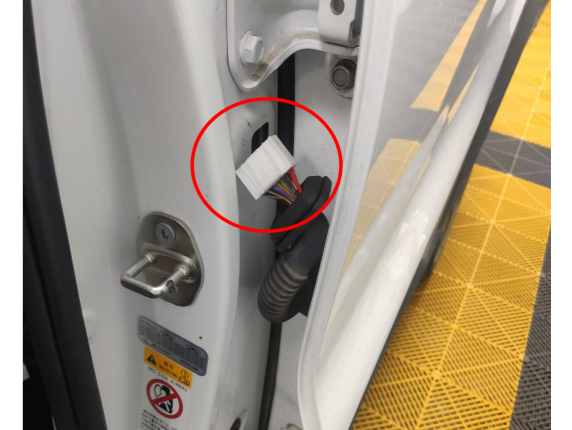
21. Connect to the B-pillar plugs.
