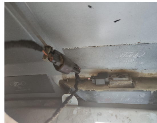
9. Connect the plugs of the lock signal harness to the plugs of original tailgate switch and the added tailgate switch.
