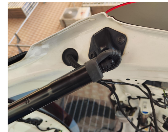
14. Thread the strut wiring harness into the tailgate and plug the hole. Both sides are the same.
