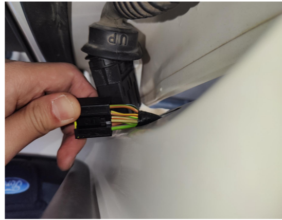
19. Connect the plugs of the power harness to the B-pillar signal plugs.
