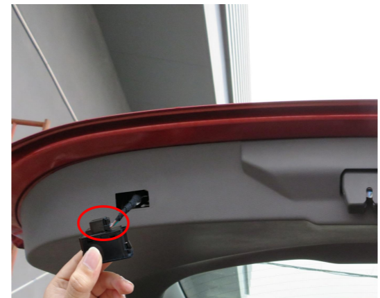
29. Reinstall all trim panels and install the added tailgate switch.
