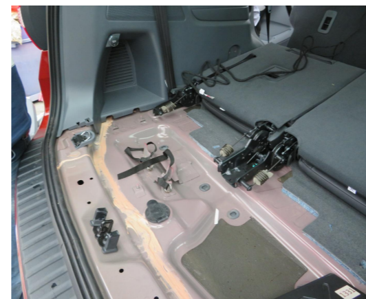
4. Take out the trunk floor mat and remove door sill panel.
