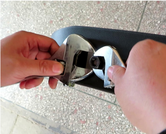
28. Open the hole (one hand secures the hole opener and the other hand turns the wrench).
