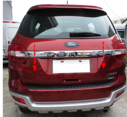
24. Press the added tailgate switch to close the tailgate once, the system completes initialization, and then test each function of the electric tailgate.
