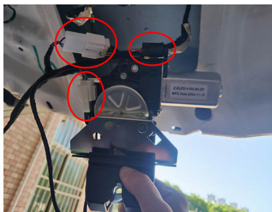
7. Connect the plugs of the lock signal harness to the plugs of the power latch.
