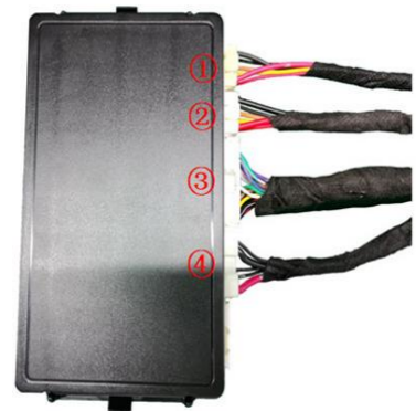
22. Insert the strut wiring harnesses ①, lock signal harness ②, and power harness ③ into the ECU in sequence.
