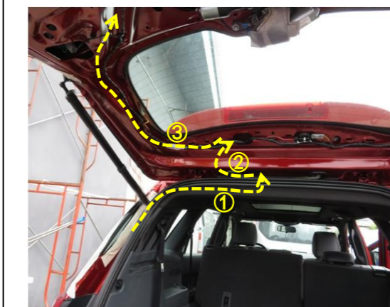
15. Thread the power harness to the tailgate.
