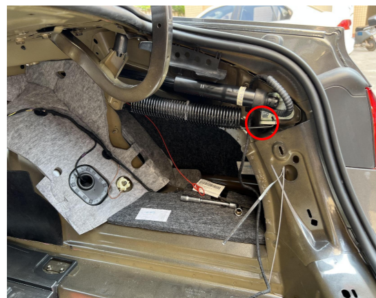
12. Hang the original springs to the middle hole of our brackets
