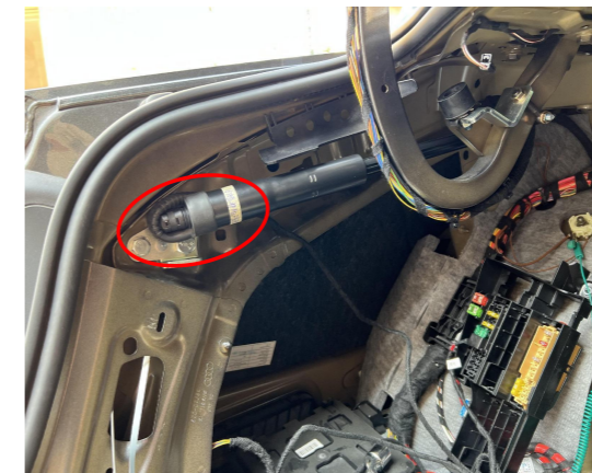
10. Install the left strut (L&R are marked as the first letter of the strut code). Pay attention to the location of rubber tube.
