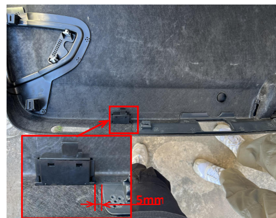
27. The location for the added tailgate switch is as shown above. Stick the hole template to the indicated location.
