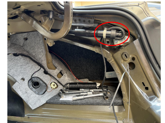
11. Install the right strut (L&R are marked as the first letter of the strut code). Pay attention to the location of rubber tube.
