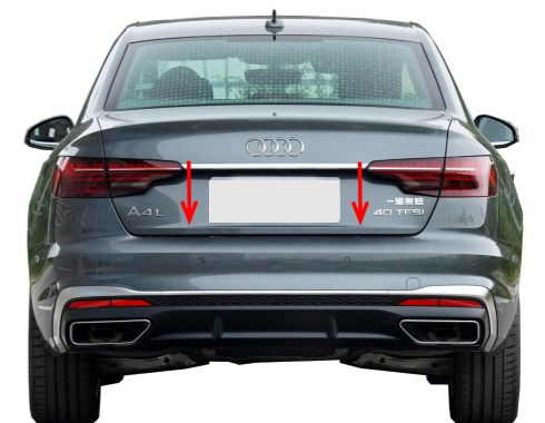
26. Press the added tailgate switch button to open and close the tailgate once for initializing the system, and then test each function of the electric tailgate.
