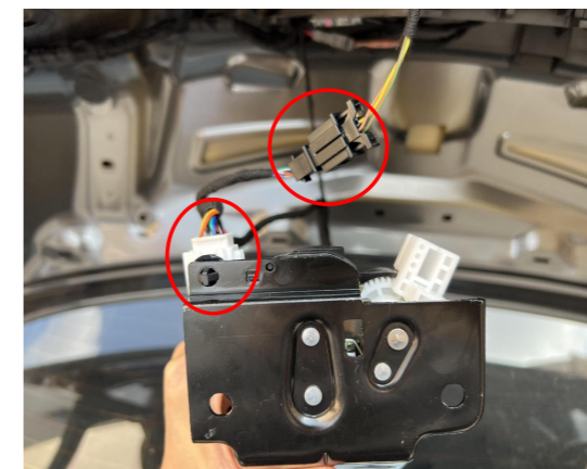
15. Connect the lock signal harness to the plugs of the power latch.
