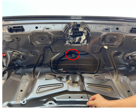
18. Connect the lock signal harness to the plugs of the original tailgate switch.
