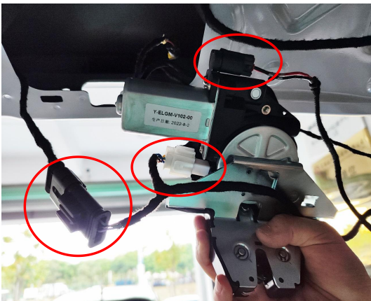
16. Connect the the plugs of lock signal harness to our power latch.
