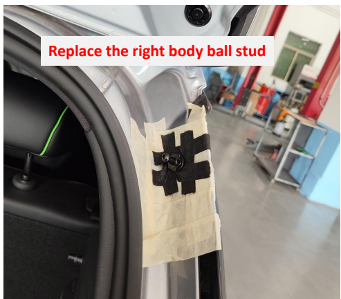
9. Replace the right body ball stud with provided one.
