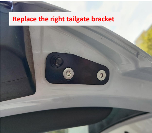
7. Replace the right tailgate bracket with provided one.
