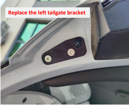
6. Replace the left tailgate bracket with provided one.
