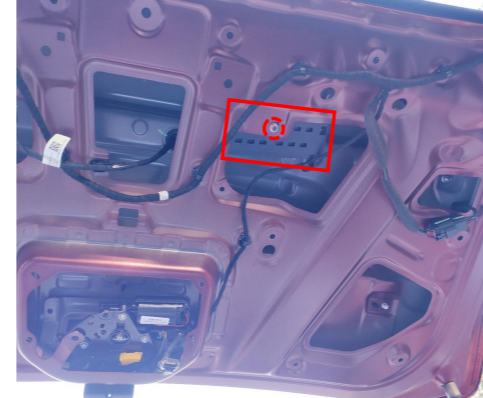
24. Remove the fastener from the indicated hole and fix the ECU bracket to the hole with a nut.
