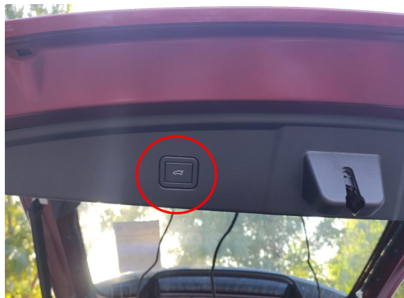
27. Reinstall all trim panels and install the added tailgate switch (remove the original small cover panel).
