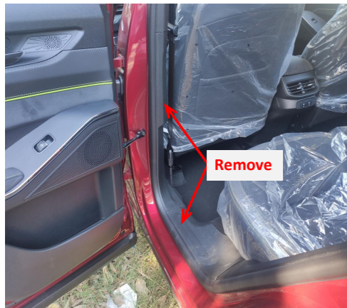
2. Remove the rear left side door sill panel and B-pillar trim panel.
