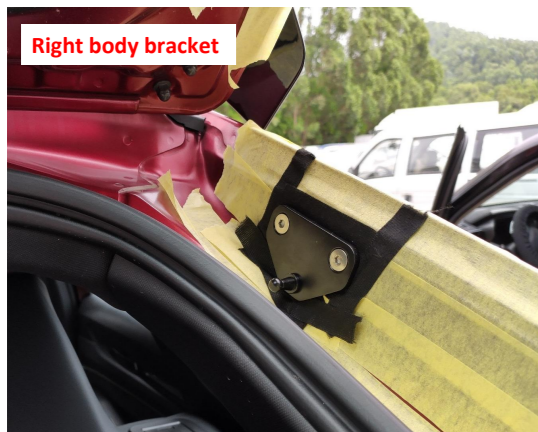
7. Replace the right body bracket.
