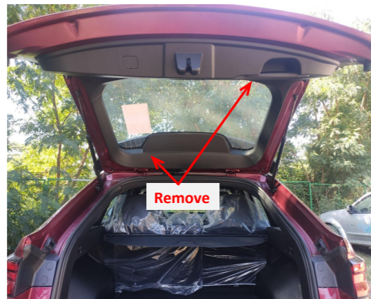
3. Remove the tailgate trim panels.
