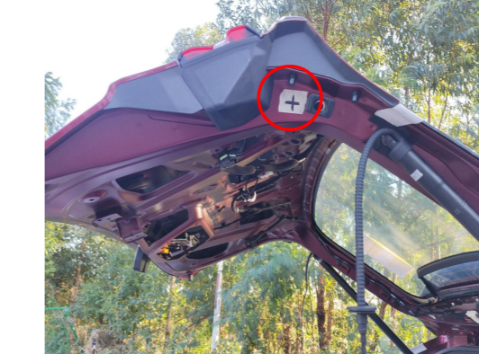
10. Drill a hole at the indicated position on the tailgate with a \phi 21\text{mm} drill bit; both sides are the same.
