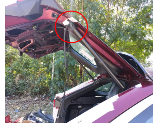
9. Install the electric struts, L on the left and R on the right (the first letter of the strut code), making sure the ends with wiring harnesses are on the tailgate.
