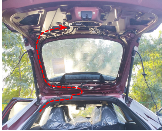
17. Thread power harness to the tailgate (wiring only, no plug or power connection).
