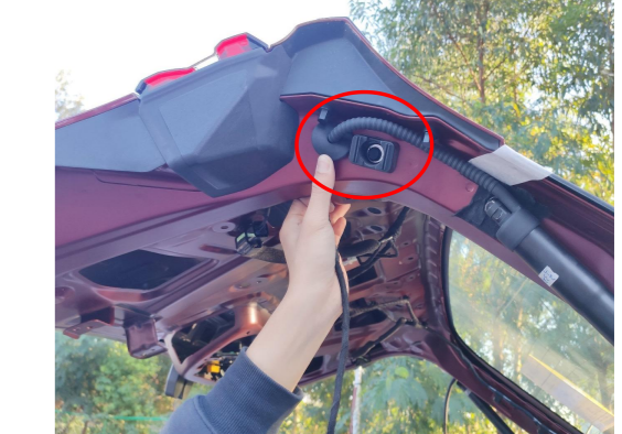
11. Pass the strut wiring harness through the indicated position into the tailgate and then plug the hole tightly; both side are the same
