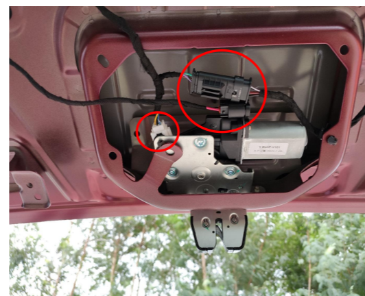
14. Connect the lock signal harness to the plugs of the power latch.
