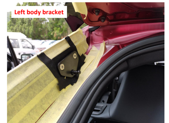
6. Replace the left body bracket.
