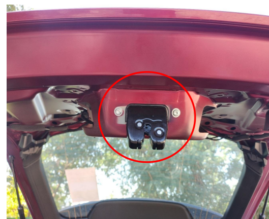
12. Remove the original latch.
