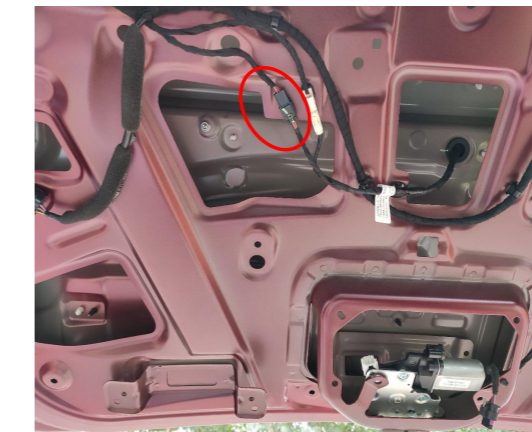
15. Connect the lock signal harness to the plugs of the original tailgate switch and the added tailgate switch.
