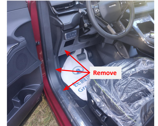
1. Remove the front left side trim panel, door sill panel and storage box.
