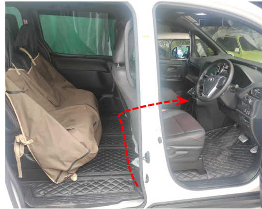
25. Route the fuse tap of the power harness from the rear seat to the front passenger seat.
