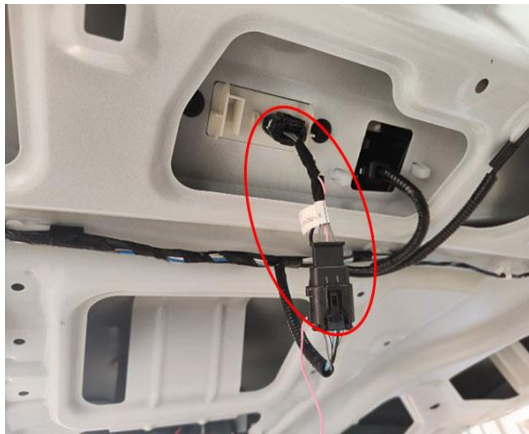
16. Connect the lock signal harness to the plugs of original tailgate switch.
