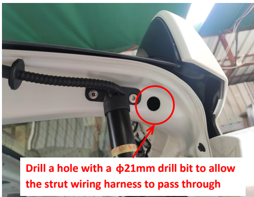
12. Drill a hole at the indicated position using a φ21mm drill bit to allow the strut wiring harness to pass through. Both sides are the same.
