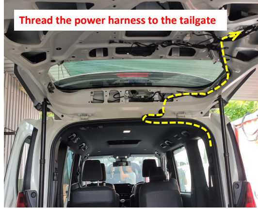
19. Thread the power harness to the tailgate.
