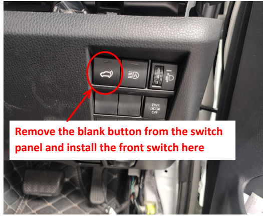
23. Remove the blank button from the switch panel and install the front tailgate switch.
