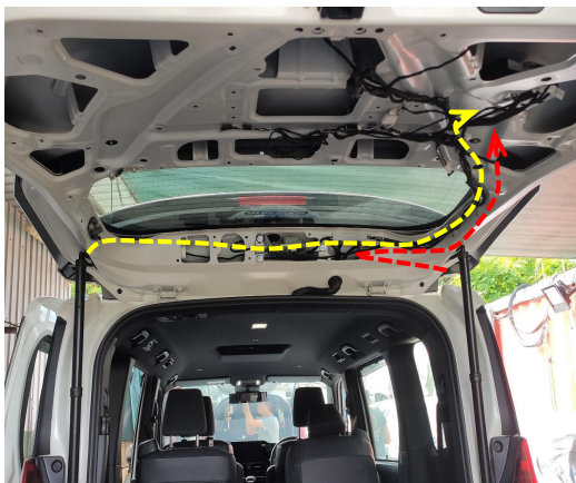
13. Route the left and right strut wiring harnesses to the tailgate.
