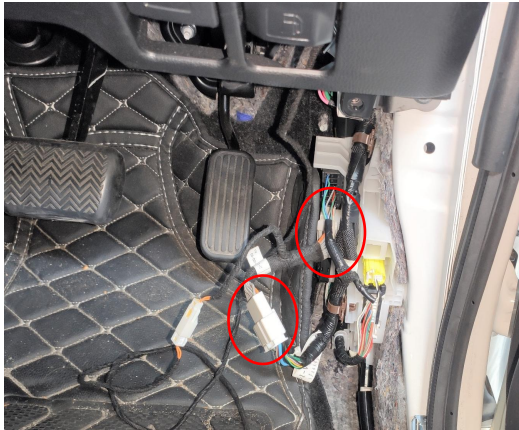
22. Connect the power harness to the signal plug and its socket beside the pedals.
