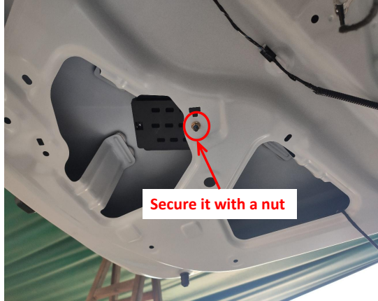
28. Place the ECU at the indicated position of tailgate and secure it with a nut.
