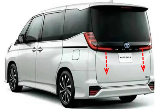
30. Press the added tailgate switch to open and close the tailgate once, the system completes initialization and then test each function of the electric tailgate.
