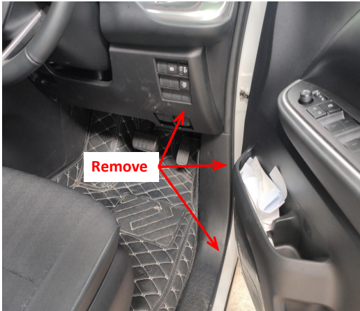
2. Remove the front right side switch panel and door sill panel.
