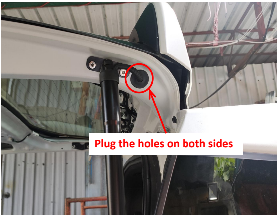
14. Plug the holes on both sides of the tailgate with hole plugs.
