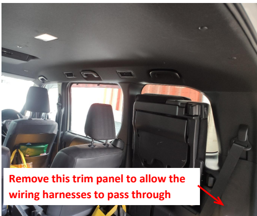
5. Remove the right side trim panel from the trunk to allow the wiring harnesses to pass through.
