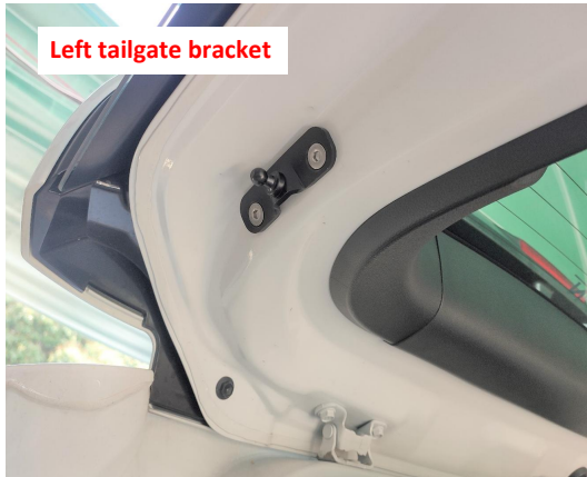
9. Install the bracket on the left side the of the tailgate.
