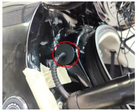
14. Plug the hole securely and leave a certain length of the rubber tube outside to prevent wire harness from being pulled.15. Remove the original screws.
