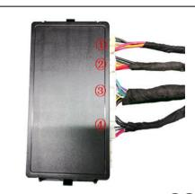
26. Insert the left and right strut wiring harnesses (1)(2), lock signal harness (3), and power harness (4) into the ECU in sequence.
