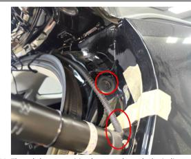
11. Thread the strut wiring harness through the indicated hole to the tailgate, the same on both sides.
