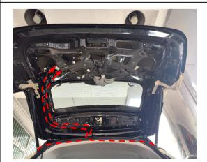
12. Route the left and right strut wiring harness to the tailgate.
