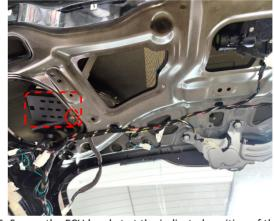
25. Secure the ECU bracket at the indicated position of the tailgate.
