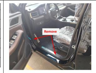
1. Remove the driver side trim panel and door sill panel.
