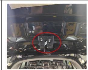
15. Remove the original latch and install the power latch with original screws
