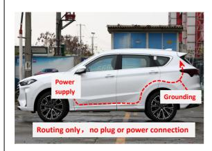
17. Connect the plugs of the lock signal harness to the plugs 18. Route the power harness (if you need to install the added ont switch route the switch wiring harness in the same way)
