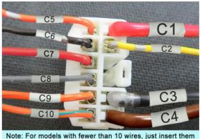
according to the corresponding label or color. 20. Insert the power harness terminals into the connector
