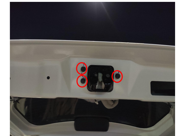
6. Remove the original latch and install our power latch.
