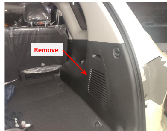
4. Remove the trim panel on the right side of the trunk to allow wiring harnesses to pass through.
