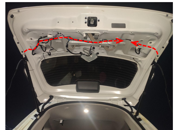
16. Route the strut wiring harnesses as shown above and then plug the holes with hole plugs.
