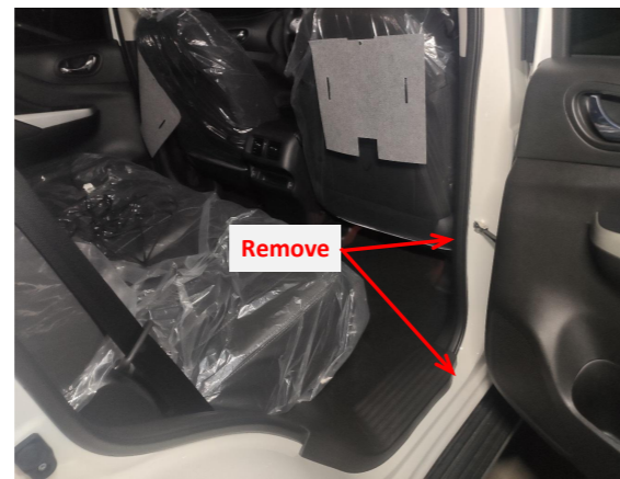
3. Remove the rear right door sill panel and B-pillar trim panel.
