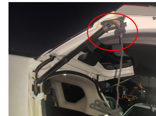
14. Install the electric struts, L on the left and R on the right (the first letter of the strut code), making sure the ends with wiring harnesses are on the tailgate.
