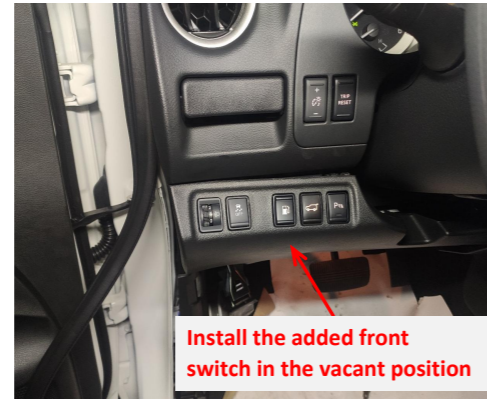
23. Replace the blank button with the front switch button and connect the other two plugs of the switch wiring harness to the plugs of the button beside it for backlight.
