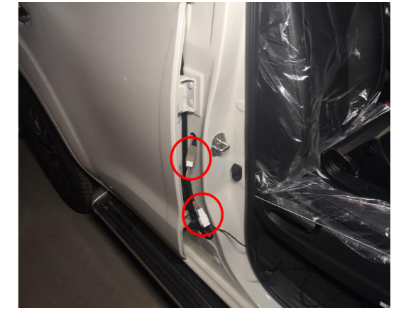
21. Connect the power harness to the signal plugs at the B-pillar on the right side of the vehicle.
