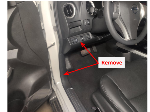
1. Remove the front left door sill panel and switch panel.
