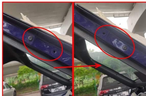
12. Remove the ball stud from the tailgate and move the plug from its original position to the threaded hole of the ball stud. Both sides are the same.
