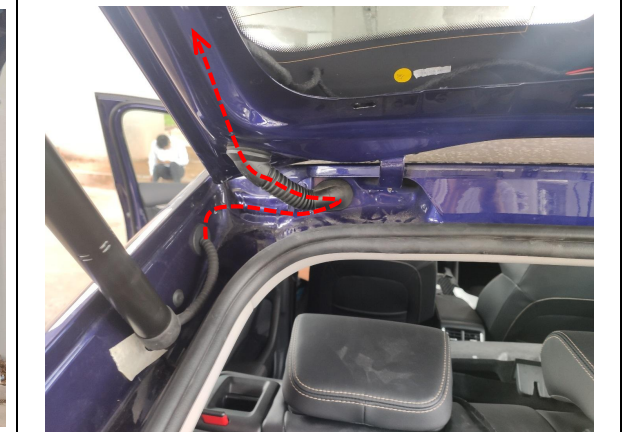
16. Thread the strut wiring harnesses through the car hole and plug the hole tightly. Both sides are the same.
