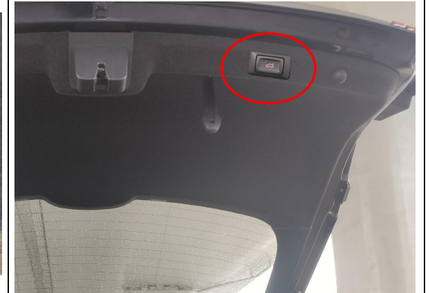
31. Reinstall all trim panels and fit the added tailgate switch in.
