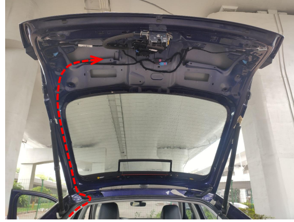
19. Thread the power harness to the tailgate.
