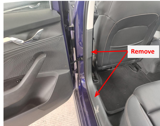
3. Remove the rear left side door sill panel and B-pillar trim panel.
