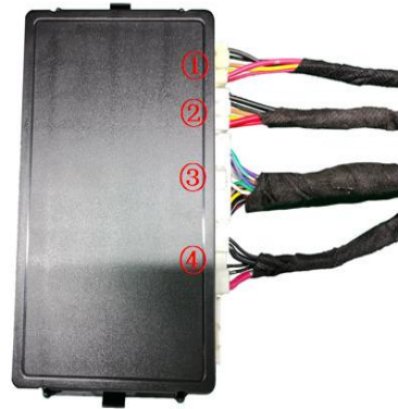
27. Insert the strut wiring harnesses ①②, lock signal harness ③, and power harness ④ into the ECU in sequence.
