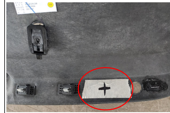
30. Align the trim panel with the enlarged hole on the tailgate and open a hole for the added tailgate switch.
