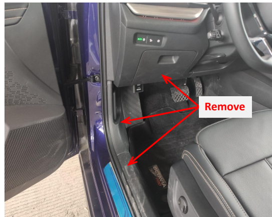
2. Remove the front left side trim panel, door sill panel and storage box.
