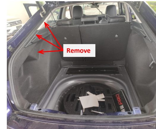
5. Take out the trunk floor mat and remove the left side trim panels.
