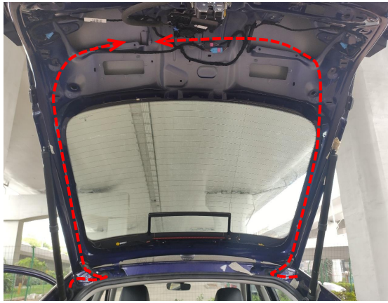
17. Route the strut wiring harnesses.
