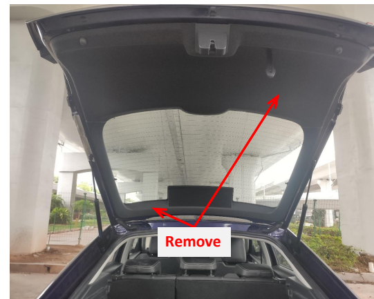
4. Remove the tailgate trim panels.
