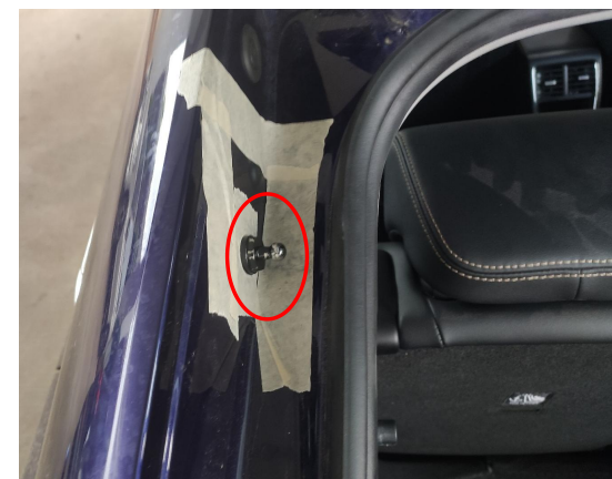
14. Replace the ball studs on the car body.
