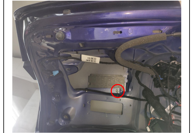
26. Secure the ECU bracket at the indicated hole on the left side of the tailgate.
