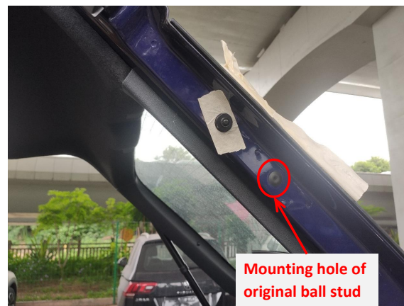
13. Install the new ball studs on the tailgate. Both sides are the same.
