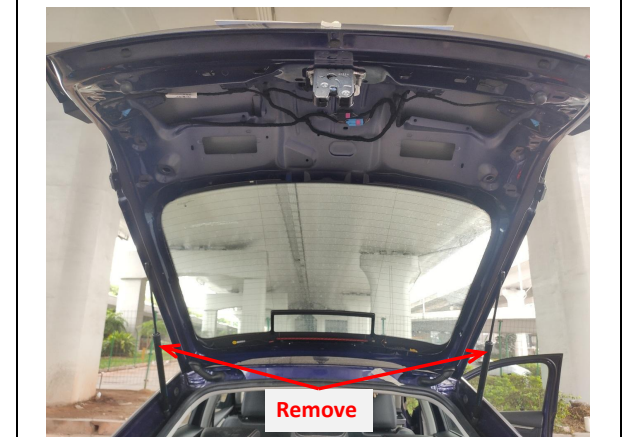
11. Remove the original gas struts.
