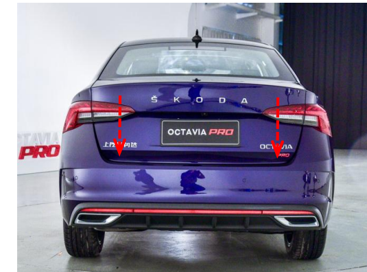
28. Press the tailgate switch buttons to open and close the tailgate once for initializing the system, and then test each function of the electric tailgate.
