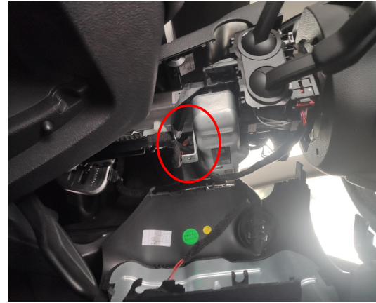
23. Connect the plugs of the power harness with the indicated signal plug and its socket.
