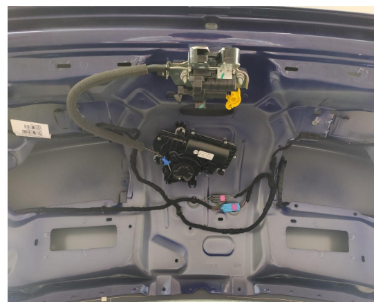
9. Remove the original latch and install our latch and actuator.
