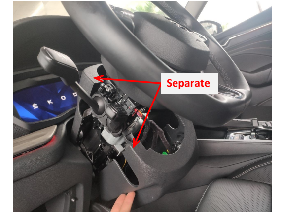
1. Separate the two steering column trim panels.
