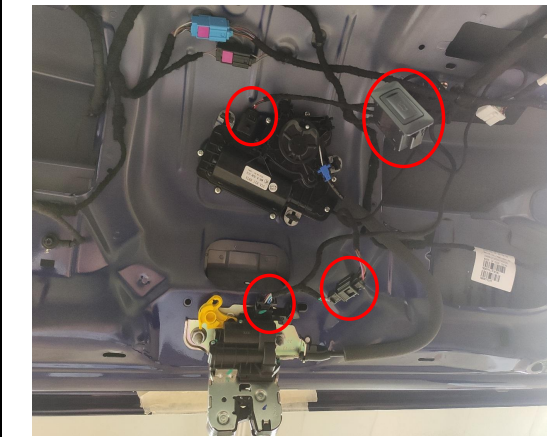
10. Connect the plugs of the lock signal harness to the plugs of the lock latch, actuator and the added tailgate switch.
