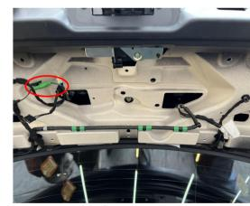
10. Connect the plugs of the lock signal harness to the plugs | 11. Connect the plugs of the lock signal harness to the plugs of the original tailgate switch.
