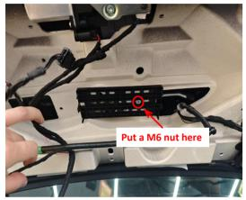
22. Install the ECU bracket with the hexalobular socket
