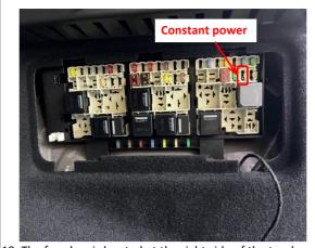
19. The fuse box is located at the right side of the trunk and 20. Plug the fuse tap into the fuse box and pay attention to the fuse slot for power supply is indicated.
