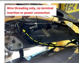
15. Thread the power harness through the indicated position under the spoiler.
