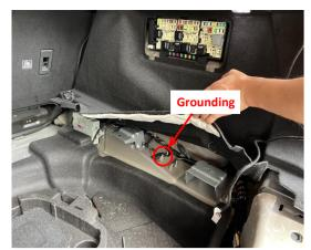
17. Ground at the indicated position on the right side of the | 18. Insert the power harness terminals into the connector trunk.
