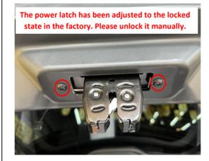
9. Install the power latch and the plastic casing.
