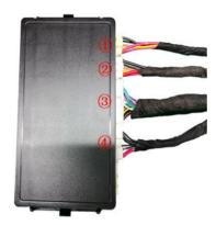
24. Insert the strut wiring harnesses (1)(2), lock signal harness (3), and power harness (4) into the ECU in sequence.
