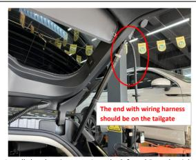
. Install the electric struts, L on the left and R on the right the first letter of the strut code).
