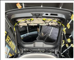
6. Route the strut wiring harnesses as indicated.
