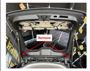
13. Remove the hinge trim panels on both sides.
