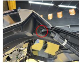
5. Thread the strut wiring harness through the indicated hole into the tailgate, the same on both sides.
