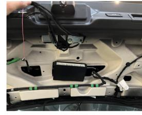
23. Fit the ECU onto its bracket.
