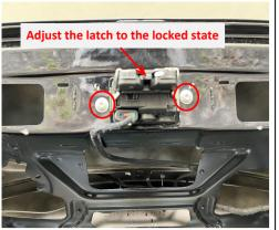
21. Install the power latch and manually adjust the latch to the locked state.
