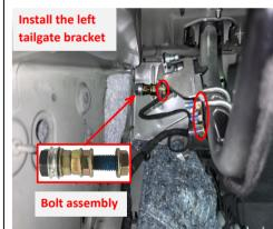
14. Tighten all the bolts with nuts.
