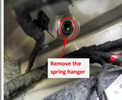
10. Remove the springs hangers on the left and right
