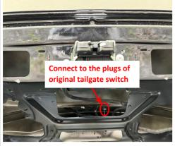
22. Connect the plugs of the lock signal harness to the plugs of original tailgate switch.
