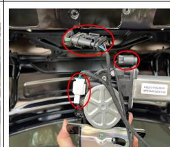
20. Connect the plugs of the lock signal harness to the plugs of the power latch.
