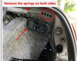
. Remove the springs on both sides. Install the right body bracket at the indicated holes and insert the screw with handle into the body from the indicated direction.
