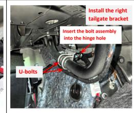
11. Install the right tailgate bracket. Insert the bolt assembly into the hinge hole first, then secure the two U-bolts on the hinge.
