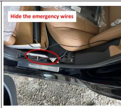
23. Wrap the two emergency wires of the latch separately with electrical tape and hide them under rear left door sill panel.
