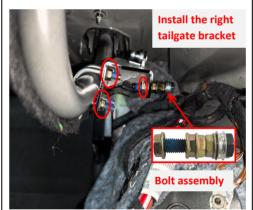
12. Tighten all the bolts with nuts.
