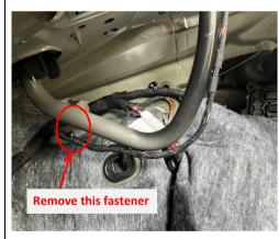
9. Remove the indicated fasteners on both sides.
