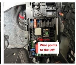
29. Plug the fuse tap into the fuse box and pay attention to the direction.
