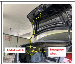
24. Route the lock signal harness along with original viring harness as indicated.
