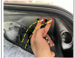
6. Thread the two screws out through the holes.
