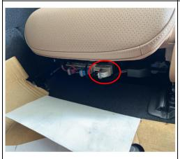
27. Connect the plugs of the power harness to the indicated CAN signal plug and its socket..
