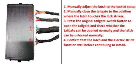
31. Insert the left and right strut wiring harnesses (1)(2), lock signal harness 3, and power harness 4 into the ECU in sequence. Tie them along with original wires.
