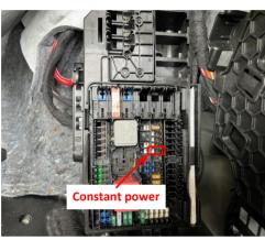
28. The fuse box is located at the right side of the trunk and the fuse slot for power supply is indicated.
