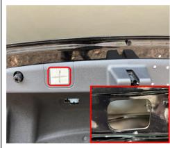
34. Stick the hole template to the indicated position and open a hole(pay attention to align with the hole on the 35. Cut off the ribs from the trim panel. tailgate).
