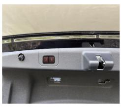
36. Install the added tailgate switch and reinstall all trim
